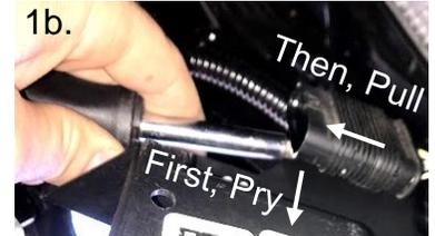
1b. Pry the detent, then remove the other connector.
