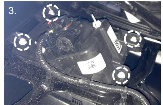
4. Remove the fog lamp. Repeat steps 2-3 for passenger side.
