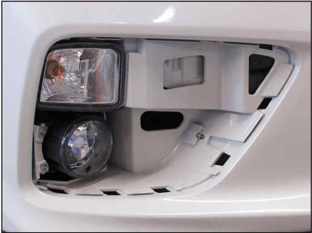
Remove the fog bezels, splash guard, or front bumper cover to gain access to the fog lights. Disconnect and remove fog lights.
