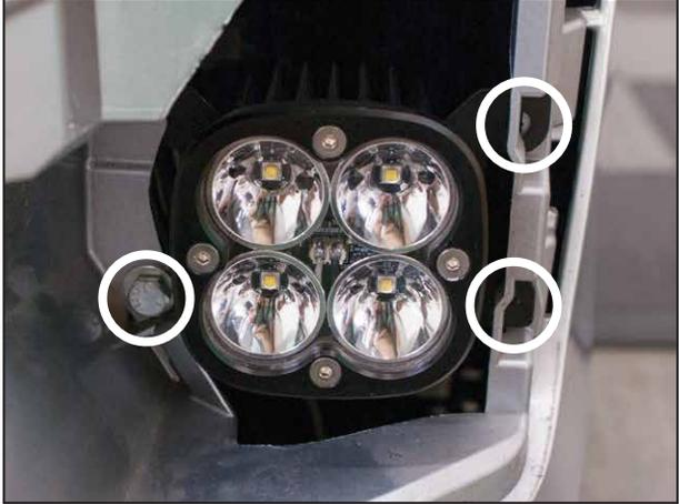
Attach Squadron assemblies to front bumper cover. Fasten with OEM hardware or included 1/4" hardware. Wire, test, and reinstall fog bezel, splash guard, or bumper cover.
