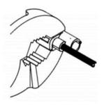
4. Route the upfitter harnesses down to the passenger side fog pocket. Attach each provided splitter to the upfitter harnesses. Attach the short lead of each splitter harness to the passenger side Squadron lights. Route the long lead of each splitter harness across the core support to the driver side fog pocket and attach to each Squadron.
