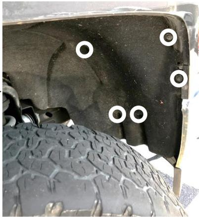
3. With the 15mm socket wrench remove the two bolts at the end of the support bar shown by the black arrows (bolts not in frame). Remove the single bolt at the other end of the support and place the bar aside. Remove the six bolts shown by the white arrows. (dashed white circle shows bolt location behind support bar)
