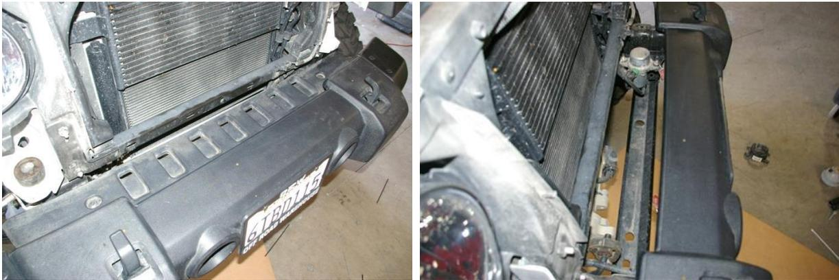
*Note: The black plastic piece can be a little tough, but once you have removed the fasteners you can twist the plastic piece and pull it out to the side.*
