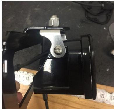
4. Install the Baja Designs Brackets and Lights into the OEM location using the factory 10mm bolts.
