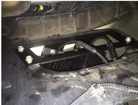
5. Plug the supplied wiring adapter into the Baja Designs Lights then into your OEM Plug.
