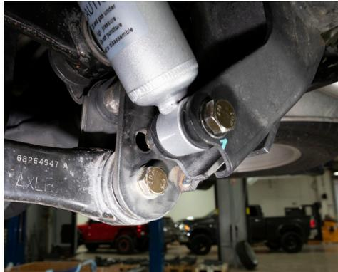
37. Torque all M16 x 2.0 nuts and bolts used to retain the control arm drop brackets to 111 ft lbs. + 110° turn.
