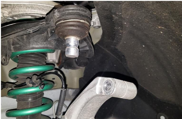
13. Remove the (4) bolts holding the upper control arm mount. It may be necessary to lift the cowl cover slightly to access the rear bolt. Do not discard the bolts. Remove the upper control arm mount and shock from the vehicle.
