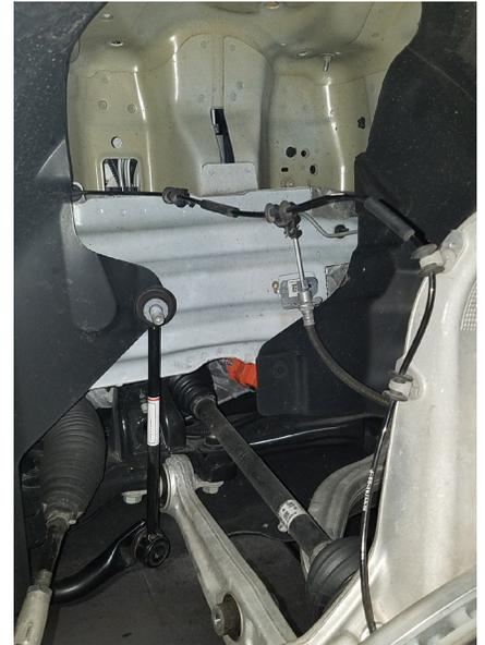
14. Remove the (3) upper shock mount nuts from the upper control arm mount and separate the shock from the upper control arm mount. Do not discard the upper mount nuts.
