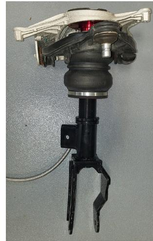
3. Install the shock and upper control arm mount assembly with the (4) previously removed bolts. Torque the larger bolts (circled in yellow) to 62Nm (45 lb.-ft.) and the smaller bolts (circled in red) to 35Nm (25 lb.-ft.).
