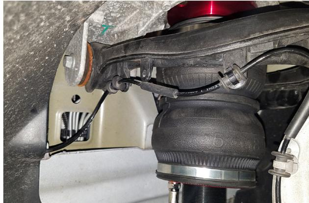
9. Replace the brake line bracket on the body. Install the nut and torque to 6Nm (4.5 lb.-ft.). (Dual motor vehicles only)
