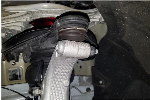
5. Raise the lower control arm and reinstall the lower shock mount bolt and nut hand-tight. Do not torque the bolt at this time.
