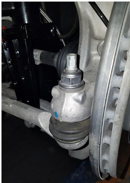
7. Reinstall the stabilizer bar end link to the strut tab and torque the nut to 98Nm (72 lb.-ft.).
