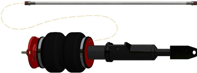
2. Using the (3) previously removed upper shock mount nuts, install the Air Lift Performance shock on the upper control arm mount and torque the nuts to 23Nm (17 lb.-ft.).
