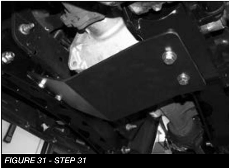
32. Proceed to torque all the differential and crossmember hardware except the lower control arm pivot bolts. These will be torqued once its on the ground.
