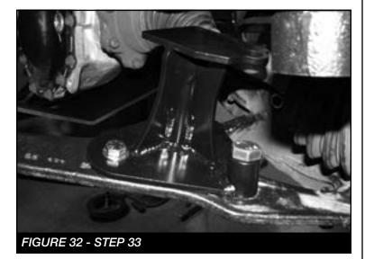
34. Install FT20775 (Bumpstop rear) on the Driver side lower control arm using the factory bolt and 1/2" X 1-1/2" hardware. Torque to 127 ft-lbs. SEE FIGURE 33
