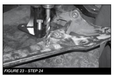
25. On the same control arm, Install the FT20775 (bump stop rear bracket) using the factory lower shock bolt. Mark the second hole. Remove bracket and drill to 1/2". **SEE FIGURE 24-26**
