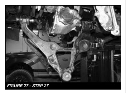
28. Install the new Fabtech spindles FT20747D & FT20747P to the upper and lower control arms. Torque to upper ball joint to 45 ft-lbs and the lower to 70 ft-lbs. **SEE FIGURE 28**
