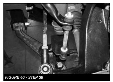
40. Locate the factory ABS module on the inside of the driver side frame. This will need to be temporarily moved to access the factory torsion bar/key crossmember bolt. Once it is moved and the bolt is accessible, remove the crossmember by removing the 2 bolts. Save hardware. **SEE FIGURES 41-42**
