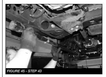
44. Torque the 9/16" hardware on the drop brackets to 184 ft-lbs. Next, re-install the factory crossmember using the factory bolts and 1/2" X 1-1/2" hardware. NOTE: The 1/2" bolts will need to be installed from the inside of the crossmember. Torque the factory hardware to 160 ft-lbs and 1/2" to 127 ft-lbs. SEE FIGURE 46
