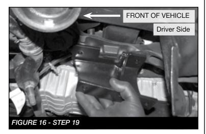
Locate and install the Fabtech Pass side Diff bracket (FT20749) to the Passenger side of the vehicles bottom factory frame mount using the factory hardware. Torque to 120 ft-lbs SEE FIGURE 17
