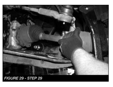
Install the hub assembly and dust shield. Torque the 4 factory bolts to 160 ft-lbs. Re-install the brake components and HUB center nut. SEE FIGURE 30
