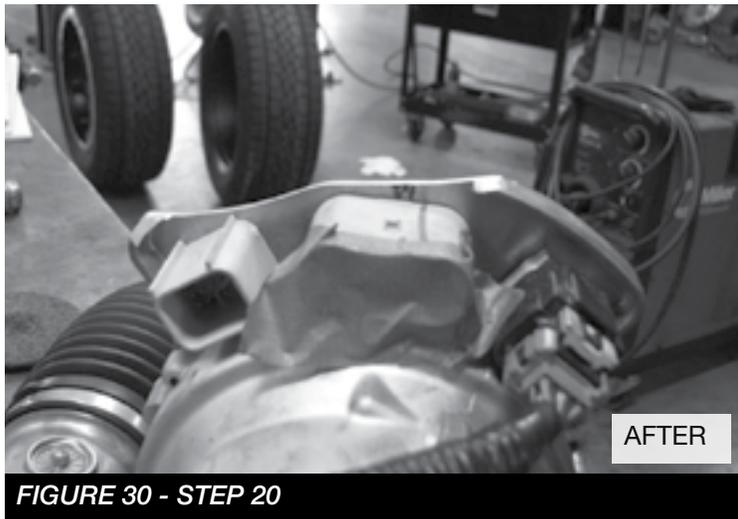
21. Disconnect the electrical connection (pass side) and the vacuum line (driver side) from the differential housing. Make sure the wire harness is completely detached from the housing. Carefully remove the differential and set aside. Retain hardware for reinstallation.
