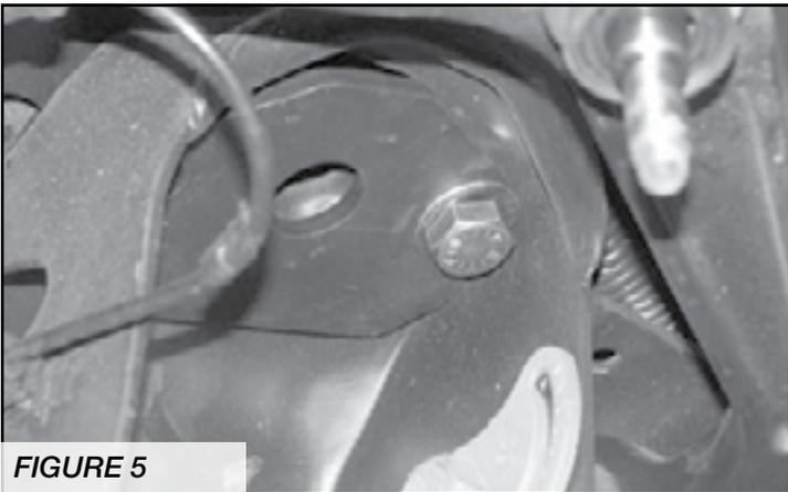
12. Install the Dirt logic front shock with the supplied bushings and washers at the upper mount then bushing and sleeve at the lower mount using the factory hardware.
