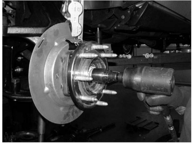
45. Install the rotor and the small bolt retaining the rotor and torque 12 ft-lbs. Install the caliper and torque to 220 ft-lbs. SEE PHOTO BELOW
