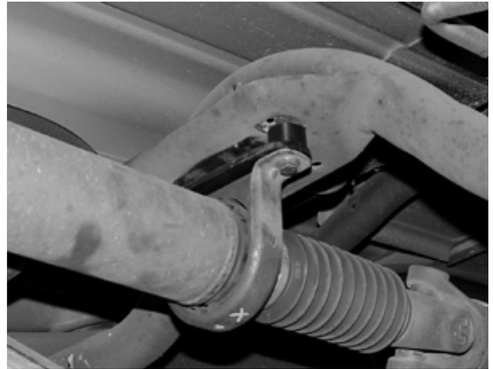
59. Recheck all bolts for proper torque. Recheck brake hoses and lines for proper clearances.
