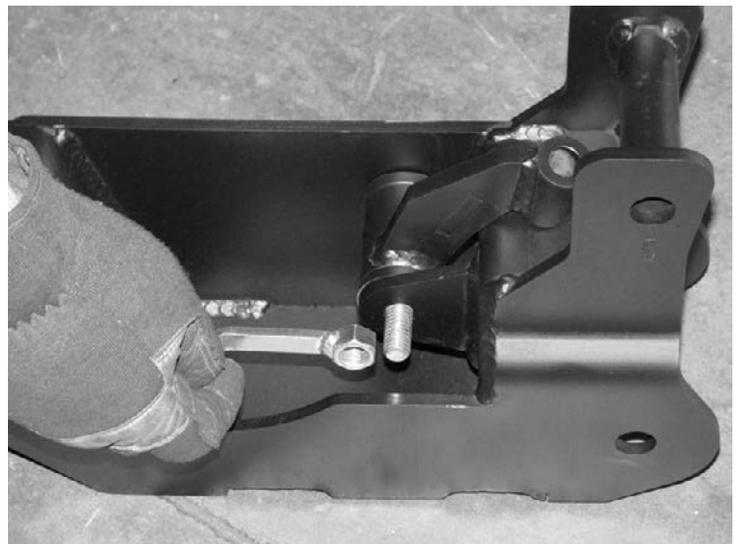
25. Install Fabtech rear crossmember (FT20475BK) using the factory control arm hardware. Leave the hardware loose at this time. SEE PHOTO BELOW
