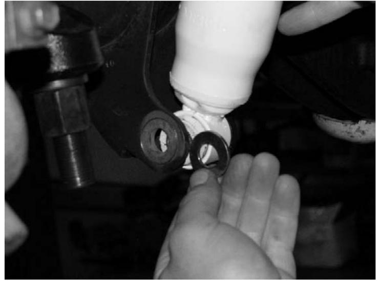
58. For vehicles with a two-piece rear driveshaft, locate and install FT20074 spacer between the carrier bearing and frame. Push out stock mounting bolts and use 3/8" x 2" bolts, nuts and washers. Torque to 30 ft-lbs. SEE PHOTO BELOW
