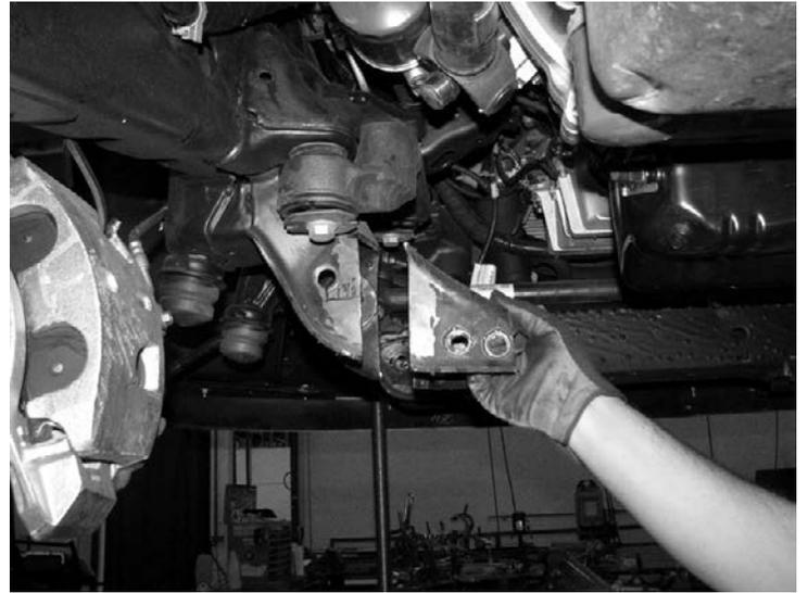
16. Locate the pass. lower control arm pocket and cut out the 3" section over the holes on the front side of the pocket. SEE PHOTO BELOW
