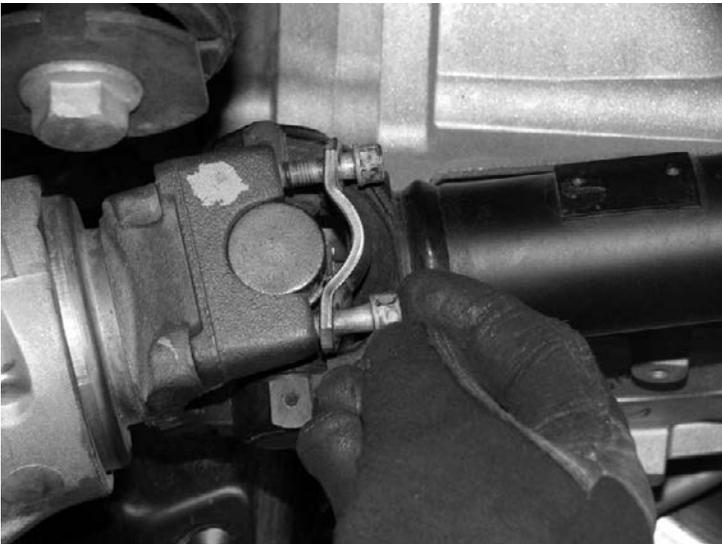
23. Locate the Rear diff bracket (FT20486). Assemble the bushings (FT1020) and the sleeve (FT181) in the barrel of the bracket. SEE PHOTO BELOW
