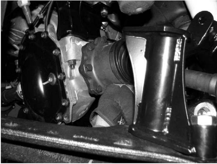
44. Locate the o-ring, dust shield and hub. Install into the Fabtech spindle. Torque the factory hub bolts 184 ft-lbs. Install the axle nut and torque to 165 ft-lbs. Replace axle nut cover. SEE PHOTOS BELOW
