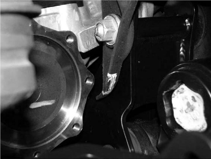
22. Reinstall the factory front drive shaft and torque to 29 ft-lbs. SEE PHOTO BELOW
