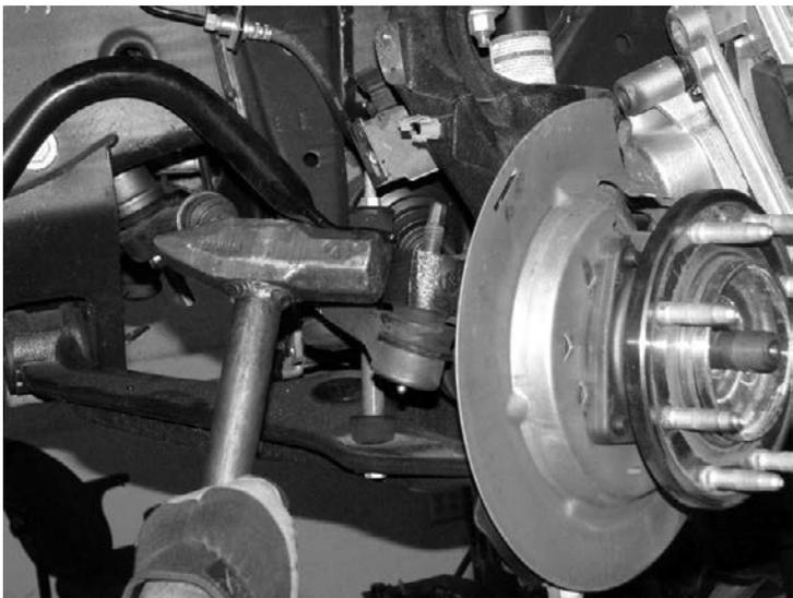
7. Remove the brake hose bracket from the top of the steering knuckle. Remove the caliper from the rotor and place above the upper control arm during this portion of the installation. . Remove brake rotor from the steering knuckle. Unbolt the wheel speed sensor connection from the hub and control arm. SEE PHOTO BELOW
