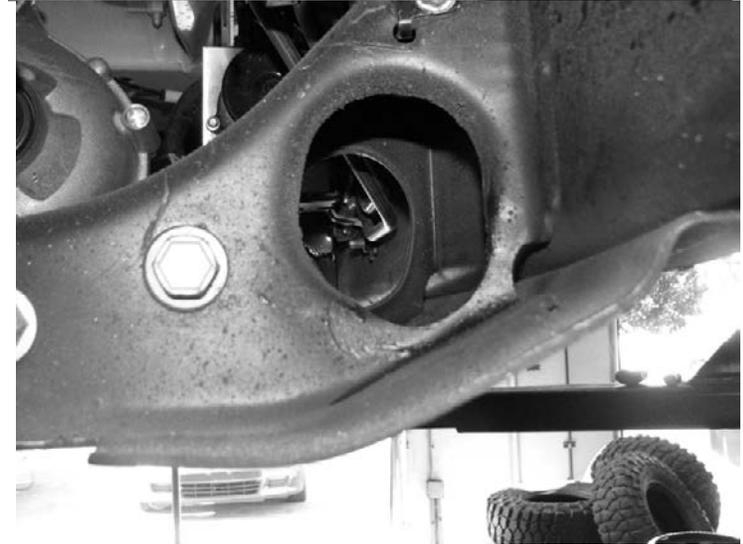
41. Locate and install the factory torsion bar through the hex in the torsion bar mount. Thread the torsion bar all the way back in the
