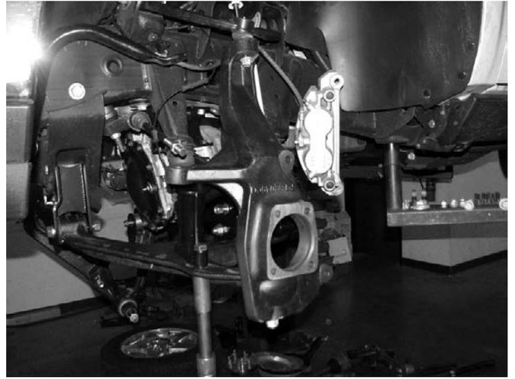
43. Locate the factory CV shaft and reinstall. Push the axle bell through the opening for the hub on the Fabtech spindle. This will locate under the shock mount on the torsion bar bracket. Bolt the flange on the CV shaft to the mating flange on the diff. Torque to 58 ft-lbs. SEE PHOTO BELOW
