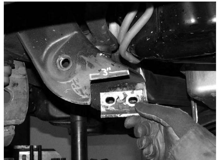
17. Locate the factory differential. Drill out the factory rear Diff mount to 1/2" SEE PHOTO BELOW
