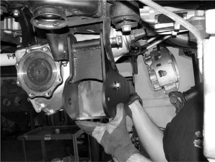
26. Attach the rear Diff mount (FT20486) to the last open mounting tab on the Factory Diff using a 1/2"-13 x 3" bolt, washers, and lock nut. Torque all the hardware to 127 ft-lbs. SEE PHOTO BELOW
