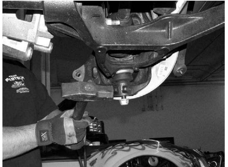
10. Disconnect CV axles from differential housing and remove axle assembly.
