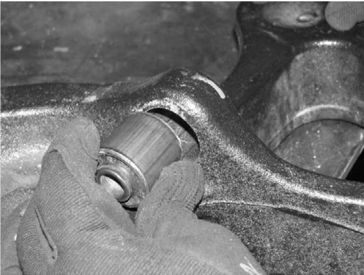
29. Locate the large aluminum RTS bushing (FT20483) and install it into the front side of the torsion bar socket in the lower control arm. SEE PHOTO BELOW
