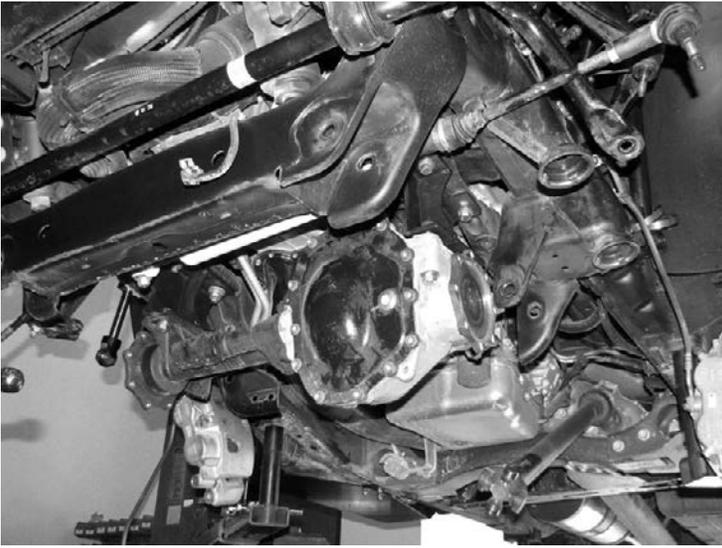
21. Check this area of the frame after installing the Diff. You may need to add a small amount of clearance for the CV. SEE PHOTO BELOW
