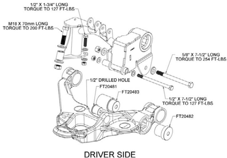
30. Locate the medium aluminum RTS bushing (FT20482) and install it into the back side of the torsion bar socket in the lower control arm. SEE PHOTO BELOW
