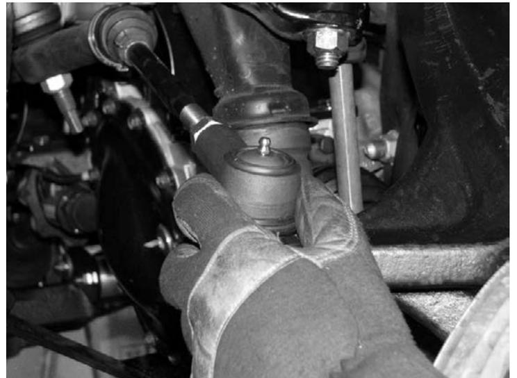
48. Insert the tie rod into the spindle and torque to 60 ft-lbs.
