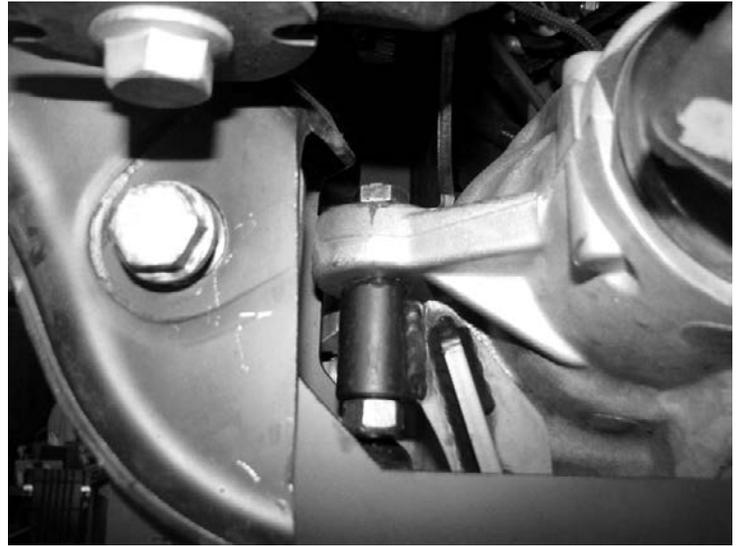
27. Locate the front crossmember (FT20474BK) and install into the factory pockets using the factory hardware. Leave the hardware loose at this time. SEE PHOTO BELOW
