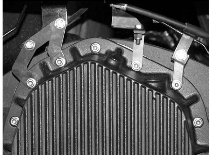
Install the E brake drop bracket (FT20511) on the driver side rear of the vehicle. Drill and install the 5/16" sheet metal bolt to lock the part in place. Use a 5/16" bolt, nut and washers to attach the brake cable to the Fabtech bracket. SEE PHOTOS BELOW
