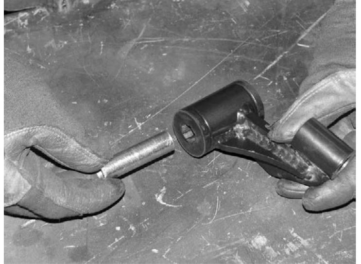
24. Install the Rear Diff bracket (FT20486) into the mount on the rear crossmember (FT20475BK). Use the 1/2"-13x4" bolt and the FT30201 nut tab to secure the bracket to the cross member. Leave loose. SEE PHOTO BELOW
