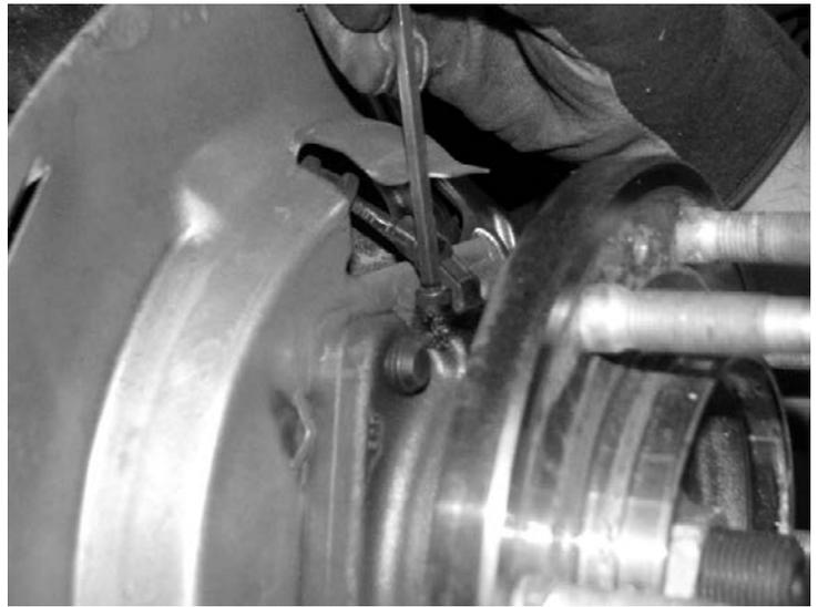
8. Remove axle nut, washer and the 4 hub bolts on backside of knuckle. Remove bearing hub assembly including O ring from knuckle. Retain parts and hardware for reinstallation.
