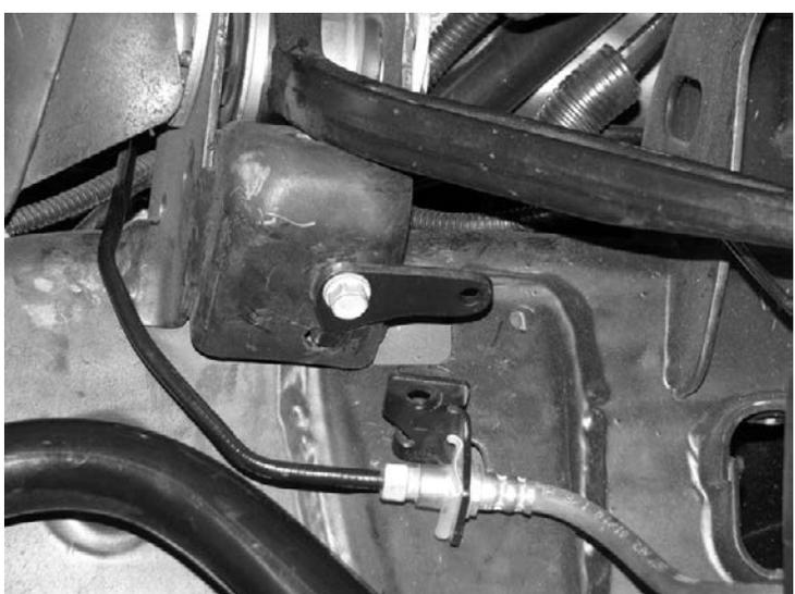
47. Remove the factory brake line bracket by either carefully cutting it off or bending it apart. Next, Install the front brake line extension bracket (FT20520) with the factory hardware and supplied 5/16" hardware. Clamp the ABS and brake line to the spindle using the supplied adel clamps and 1/4" bolts. SEE PHOTOS BELOW
