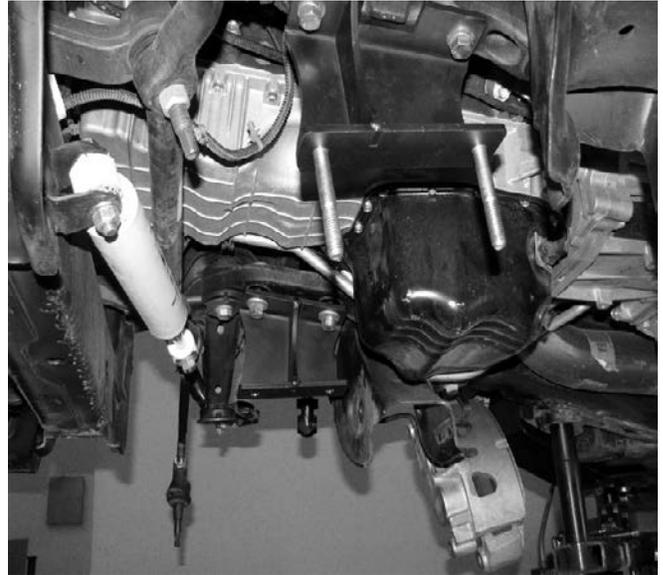
20. Locate the stock differential and reinstall with the 2ea 1/2"-13 x 3-1/2" bolts, washers and lock nuts on the driver side and the 2-1/2"-13 x 1-1/2" bolts, washers and lock nuts on the pass side. Torque all the bolts to 127 ft-lbs. SEE PHOTOS BELOW
