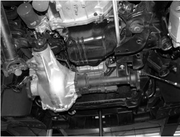
15. Locate the driver side lower control arm pocket closest to the rear of the vehicle, measure 1-3/8" from the pivot hole of the pocket and mark a vertical cut line around entire pocket. Using a Sawzall or die grinder cut the backside of the pocket and rear differential crossmember off the frame. SEE PHOTO BELOW
