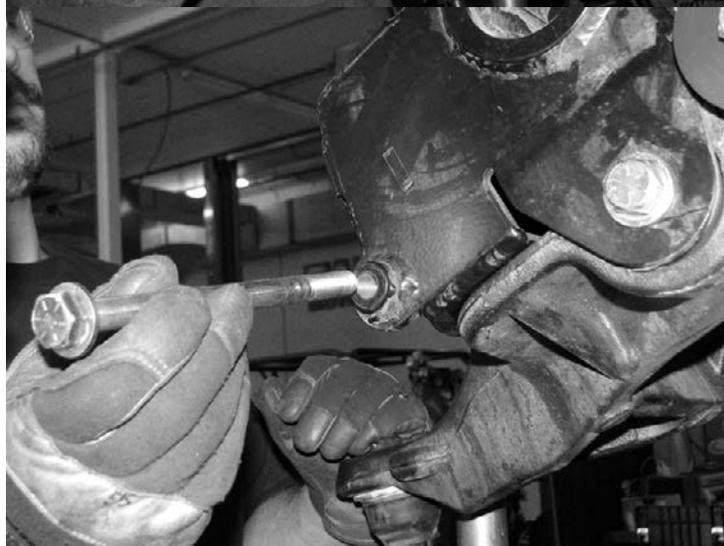
35. Locate the Torsion Bar mount for the Driver side lower control arm (FT20806). Install the torsion bar relocater to the arm using the supplied hardware  $\frac{1}{2}$ "-13 x 7-1/2",  $\frac{1}{2}$ "-13 x 1-3/4", 5/8"-11 x 7-1/2", M18-2.5x70mm., washers and lock nuts. Reference the diagram above step 29 for all the torque specifications for the torsion bar bracket. SEE PHOTO BELOW
