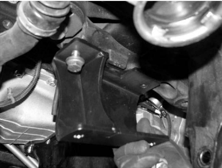
19. Locate and install the Fabtech Pass side Diff bracket (FT20477) to the bottom of the factory frame mount using the factory hardware. SEE PHOTO BELOW
