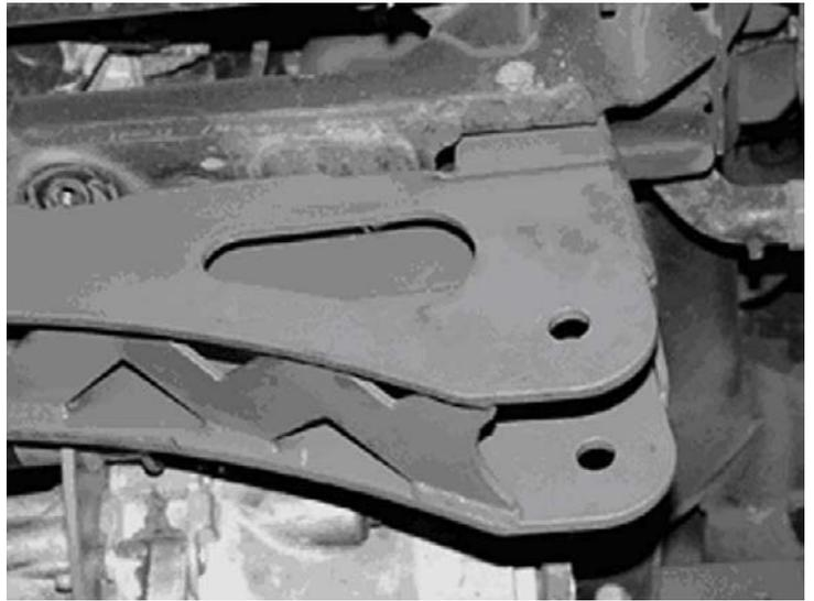
26. Position the front differential urethane bushing mount into the front crossmember tabs. Locate and install the differential skid plate around the differential housing bushing using 9/16"x 5" bolt, nut and washers from hardware kit FT20076. Leave loose.
