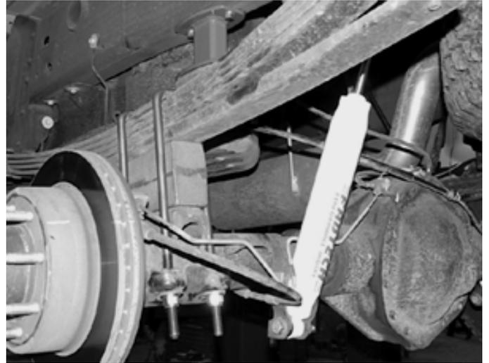
48. Install Fabtech shock part number FTS7333 (not included) with the factory hardware and torque bolts to 127 ft-lbs.
