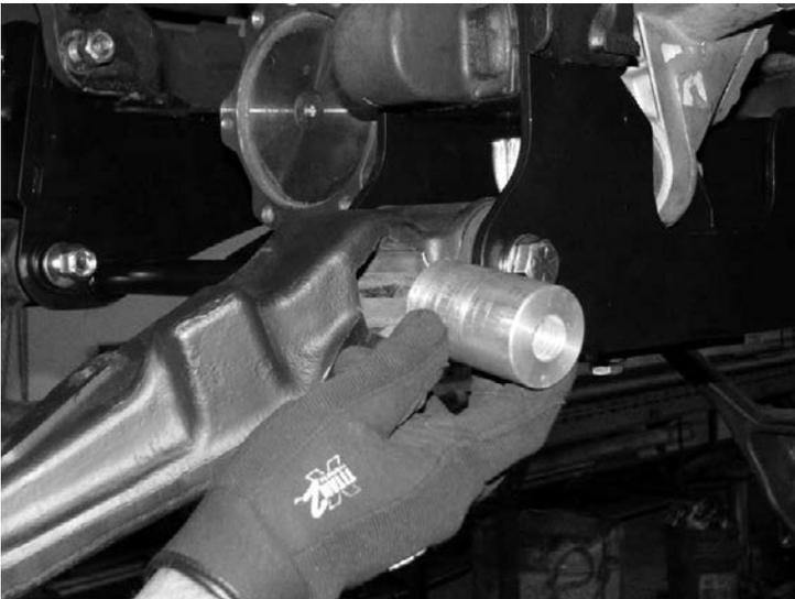
33. Locate the Torsion Bar Relocator FT20455BK and install it on to the lower control arm using the factory shock mount bolts and the supplied 3/4"-10 x 4-1/2" hardware. Torque the factory bolts to 58 ft-lbs and the 3/4 to 450 ft-lbs. SEE PHOTOS BELOW
