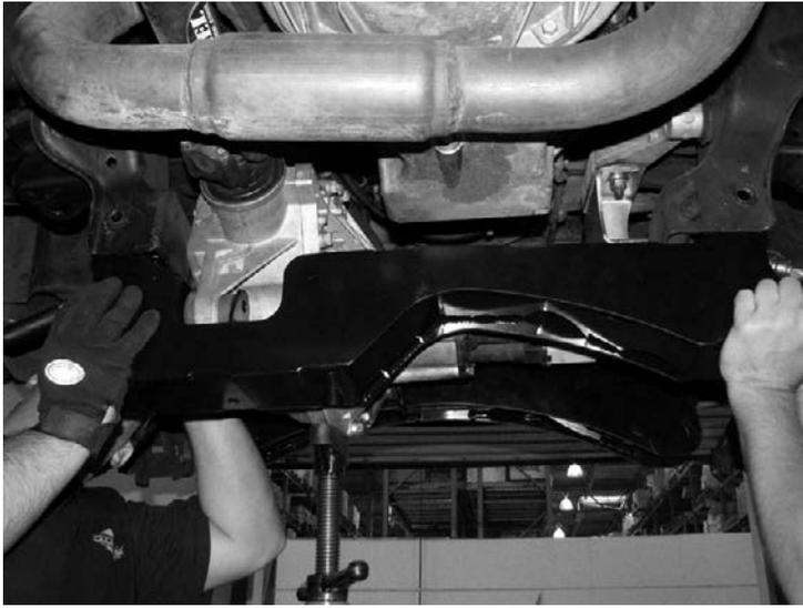
24. Locate and install the Fabtech Passenger side Diff bracket FT20061 to the bottom of the factory frame mount, with the wide end of the bracket to front of the vehicle. Attach using the stock hardware. Torque to 70 ft-lbs. SEE PHOTO BELOW.
