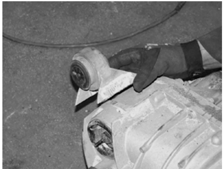
19. **On some model trucks**, the differential has a small area the needs to be sanded down level to allow the supplied Drv. Diff bracket to fit flush against the diff. Using a sanding disc, sand the differential as shown in the following two pictures. **USE CARE TO NOT SAND TOO FAR, YOU WILL ONLY NEED TO APPROX. 1/4"**. SEE PHOTO BELOW.
