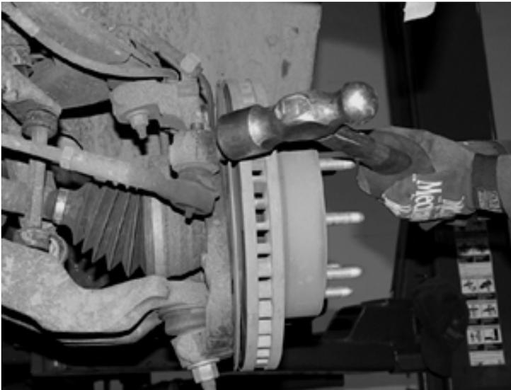
8. Remove the brake hose bracket from the top of the steering knuckle. Unplug the ABS brake connection from the frame and control arm. Remove the caliper from the rotor and place above the upper control arm during this portion of the installation.
