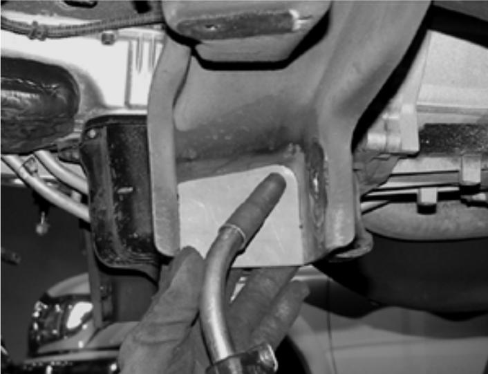
18. Locate the mounting bushing eye on the upper front side of the differential housing and mark the housing with a cut line flush to the housing. Using a sawzall cut the entire ear off the housing. Take care not to cut into the flat portion of the housing. SEE PHOTO BELOW.
