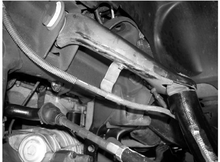
38. Reinstall the torsion bars by pulling them through the torsion bar relocator bracket and then sliding it back into the factory torsion key. Set the torsion adjuster to the premeasured height. SEE PHOTO BELOW.
