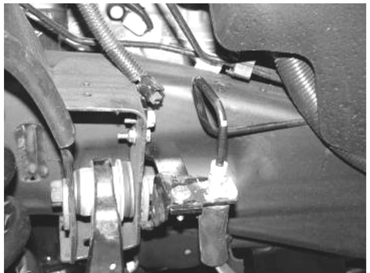
38. Re-route the brake hose and the ABS Line to the steering knuckle using the adel clamp to the back of the steering knuckle and attach with 1/4" x 3/4" bolt and washer. Torque to 10 ft lbs. Route the ABS line next to the brake hose. Re-connect the ABS line to the harness in the wheel well. Using provided plastic tyrap secure line to the hose and away from the tire and wheel. SEE PHOTO BELOW
