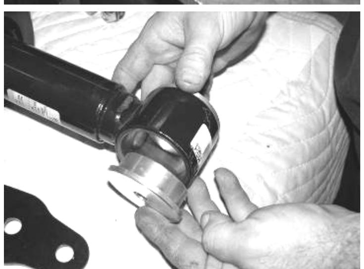
26. Locate Box 3 FTS21042BK which has FT20339 Shock Mount to Arm, FT20323 Shock Extensions, FT20568 Shock Brackets, FT20342 (**non auto-ride**) or FT20351 (**auto-ride**) Aluminum Bushings , Hardware Kit FT20295, FT1036 Bushings, and FT148 Sleeves. Using a press, press the bushings and sleeves (**Important:** must use the provided lube) into the shock extension. Insert the Aluminum Bushings into the bottom of the factory shock. SEE PHOTOS IN NEXT COLUMN
