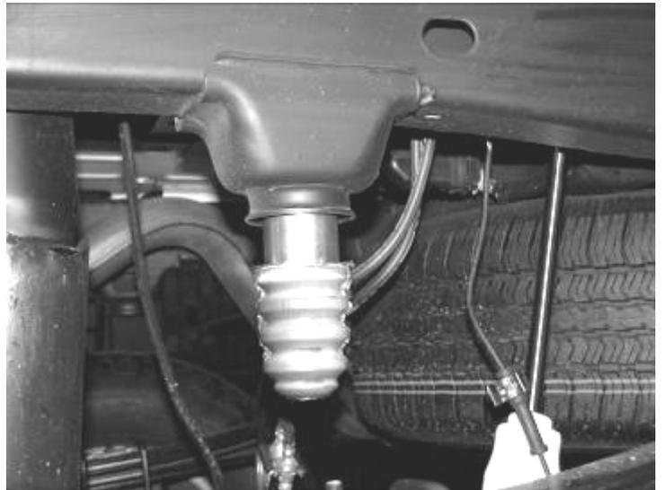
47. Locate FT20349 Brake Line Bracket and the supplied 5/16" hardware. Attach the new bracket to the differential and attach the brake line to the new bracket. Torque to 20 ft lbs.
