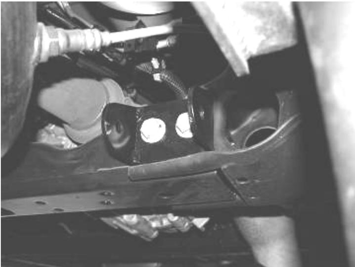
41. Locate and install the bushings into the Impact Strut bars. Attach the Impact Struts into the tabs on the back side of the lower control arm crossmember and rearward to the Impact Strut mounts using 7/16" x 3-1/2" bolts, nuts and washers from Hardware. **\*\* NOTE\*\* MAY NEED TO MODIFY EXHAUST TUBE FOR CLEARANCE ON**
