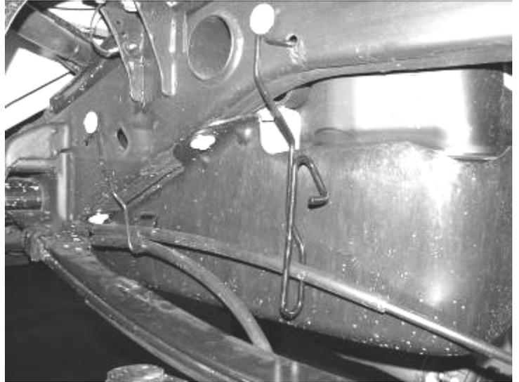
52. Recheck all bolts for proper torque. Recheck brake hoses and lines for proper clearances.
