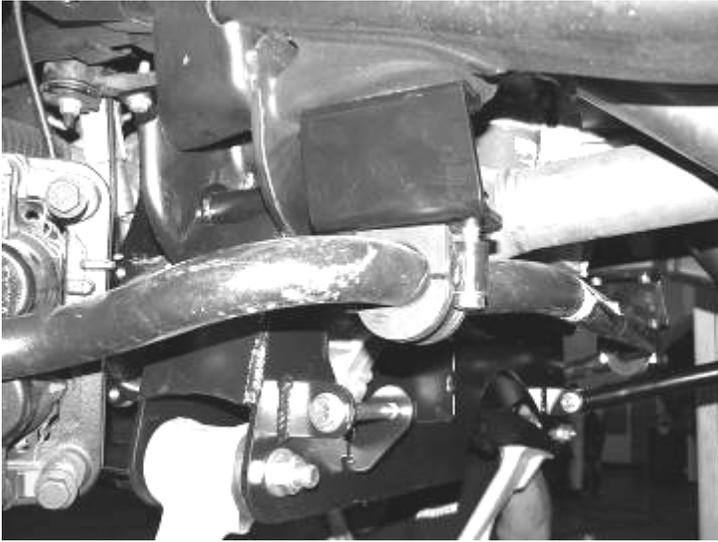
36. Locate FT20602 Sway Bar Mounts and the supplied 18mm x 50mm hardware. Position the Sway Bar Mount so that it is on the bottom of the sway bar with the SHORTER side of the mount against the stop plate end of the mount. Attach with the 18mm hardware and torque to 110 ft lbs. Locate the factory sway bar end links and attach to the new mount and the lower control arm. SEE DIAGRAM BELOW.
