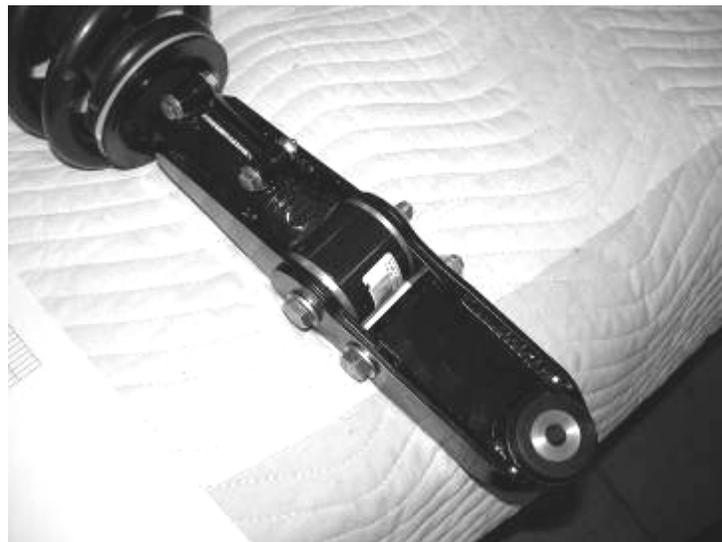
28. Locate the factory upper shock hardware. Install the shock into the factory shock bucket and leave loose. SEE PHOTO BELOW AND ON NEXT PAGE.
