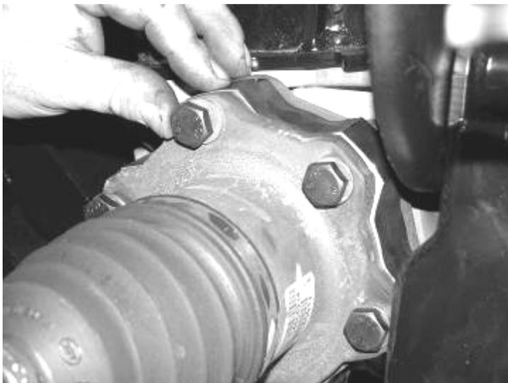
33. Reinstall the rotor and hub bearing assembly using the stock hardware and torque flange bolts to 125 ft lbs. Reinstall brake rotor and caliper. Torque caliper bolts to 30 ft lbs.
