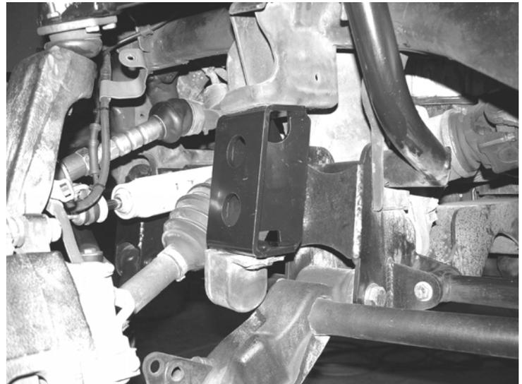
32. Locate the FT20246D & P steering knuckle and install the stock hub bearing assembly taking care to place O ring in the proper position. Apply thread lock compound to the stock hardware torque the flange bolts to 130 ft-lbs. SEE PHOTO BELOW.
