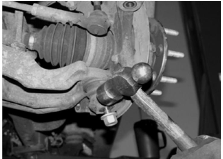
11. Disconnect CV axles from differential housing and remove axle assembly.
