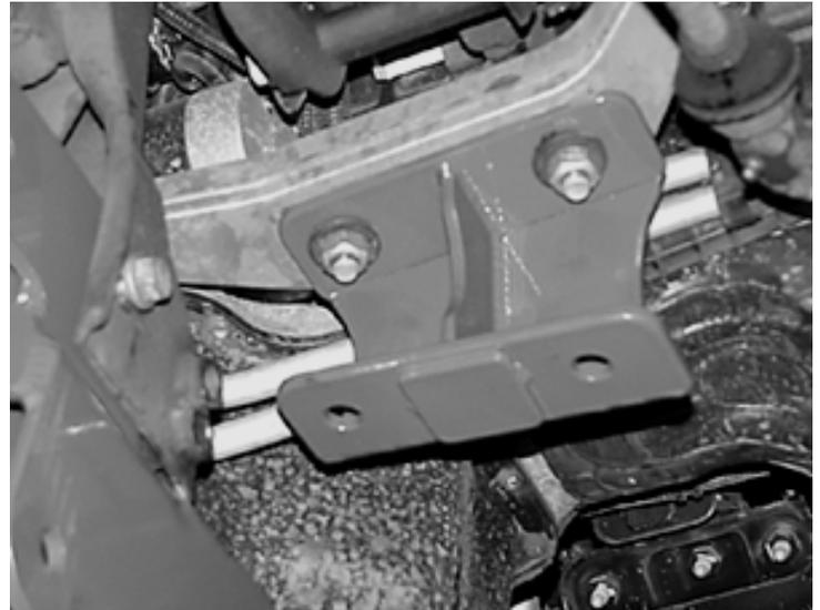
24. Place the differential housing into the Fabtech rear crossmember using the stock hardware on the driver side and 9/16"-12 x 1-3/4" bolts, nuts and washers on the passenger side from hardware kit FT20076, leave loose. SEE PHOTO BELOW
