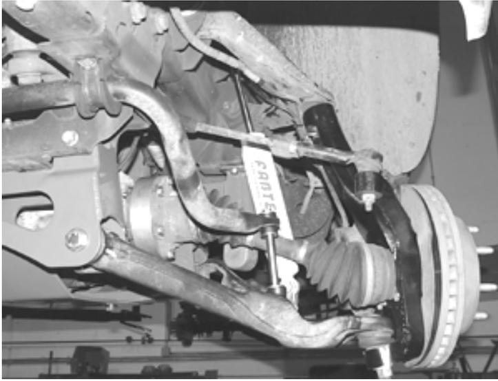
40. Recheck all bolts on front end for proper torque before proceeding to next step.
