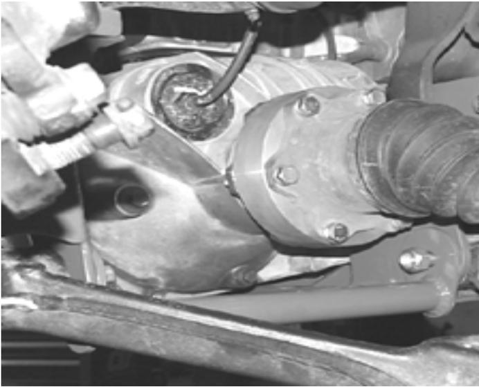
35. Install Fabtech shock part number FTS7191 (not included) using factory hardware. Torque the upper stem bushing to 15 ft-lbs and the lower bolt to 35 ft-lbs.
