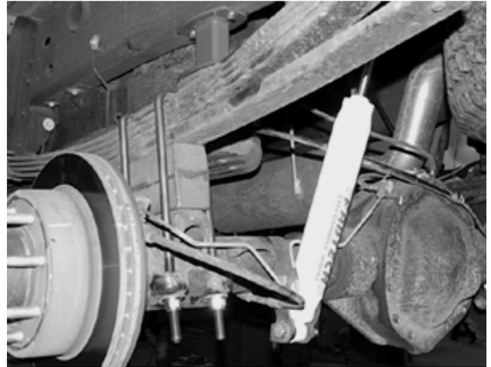
52. Install Fabtech shock part number FTS7333 (not included) with the factory hardware and torque bolts to 90 ft-lbs.
