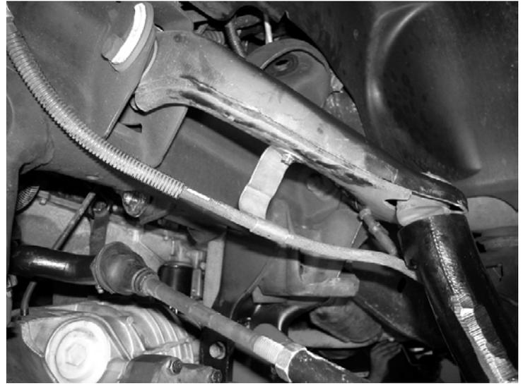
37. Reinstall brake rotor and caliper. **Note: If your brake caliper cage has the boss shown below, it must be ground / sanded flush with the cage before mounting the calipers. SEE PHOTOS.** Torque caliper bolts to 70 ft-lbs. Route the brake hose and ABS line to the steering knuckle using the factory steel guide clamp to the side of the steering knuckle and to the control arm bracket with 1/4" x 1" bolts, nuts and washers. Torque to 5 ft-lbs
