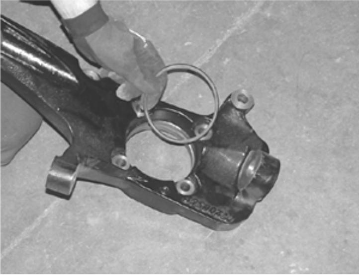
33. Attach the steering knuckle to the upper control arm and to the lower control arm using the stock hardware. Torque the upper ball joint to 35 ft-lbs and lower to 70 ft-lbs. Reattach the tie rod and torque to 30 ft-lbs.
