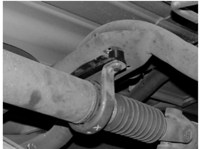
54. Recheck all bolts for proper torque. Recheck brake hoses and lines for proper clearances.
