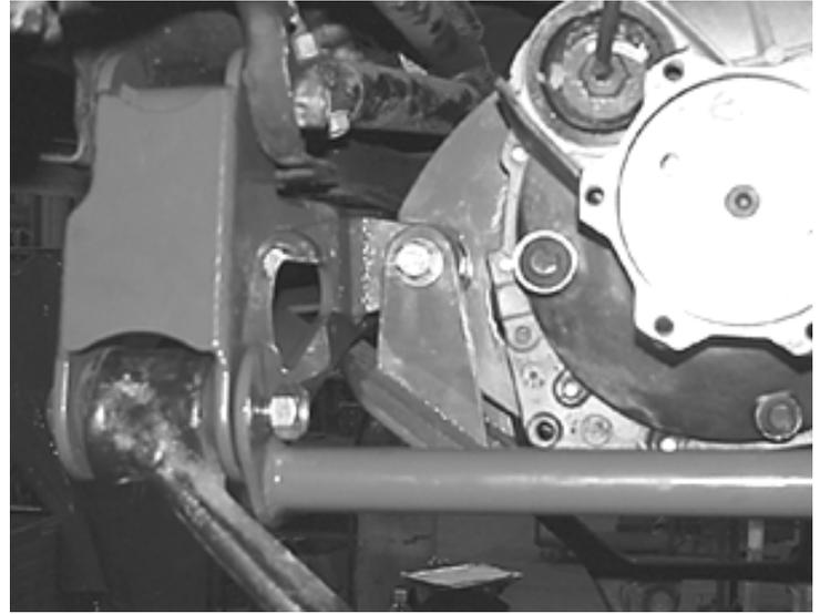
29. Using  $1/2$ " x 1-1/4" Bolt, nut and washers attach the rear of the skid plate to the bottom of the rear crossmember and torque to 50lbs.
