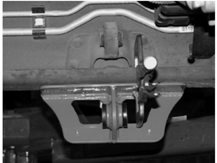
46. Re install the driver and passenger side torsion bars with the factory torsion bar crossmember into the new Torsion Bar mounts using the factory hardware and torque to 70 ft-lbs.
