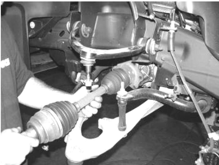
8. Remove the lower control arms from the frame and retain with the hardware for reinstallation. SEE PHOTO IN NEXT COLUMN.
