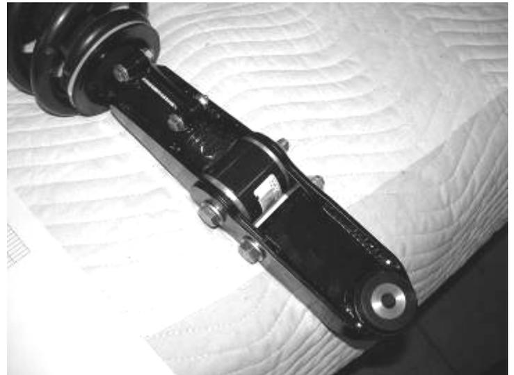
28. Locate the factory upper shock hardware. Install the shock into the factory shock bucket and leave loose. SEE PHOTOS BELOW AND ON NEXT PAGE.
