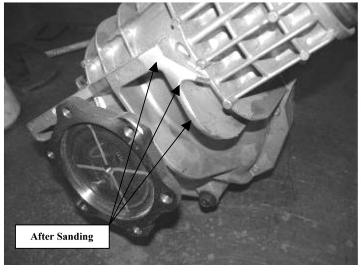
**USE THESE MEASUREMENTS AS A STARTING POINT AND CLEARANCE THESE AREAS AS NEEDED FOR PROPER FITMENT OF THE DIFFERENTIAL**
