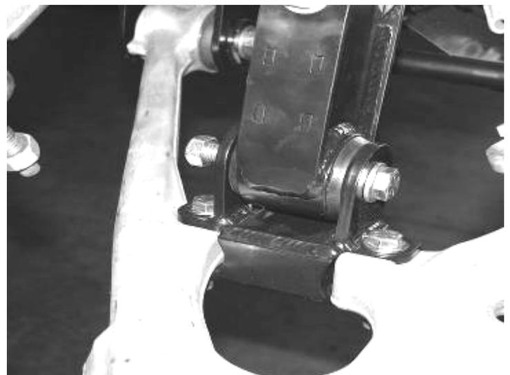
30. Locate the steering knuckle FT20276D and FT20276P. Attach the lower control arm to the knuckle using the stock hardware and torque to 70 ft lbs. Attach the upper control arm to the new knuckle using the factory hardware and torque to 35 ft lbs.
