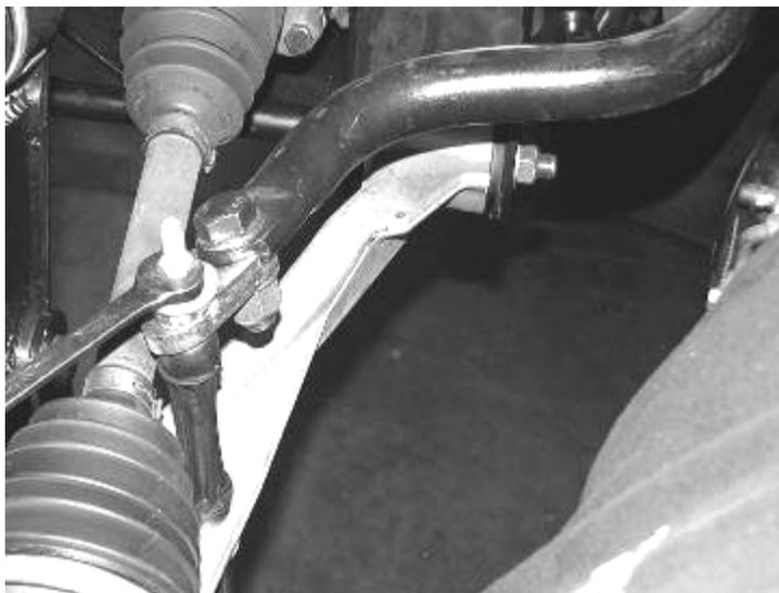
37. Locate FT20313 (drv.) FT20314 (pass) Brake Line Bracket and 1/4" x 3/4" hardware. Position the new bracket into the factory brake line bracket location and attach with the factory hardware and the 1/4" hardware. Attach the factory brake line bracket to the new Fabtech bracket. Carefully bend the hard brake line and attach with the supplied 1/4" hardware. Torque to 10 ft LBS. SEE PHOTOS IN NEXT COLUMN.
