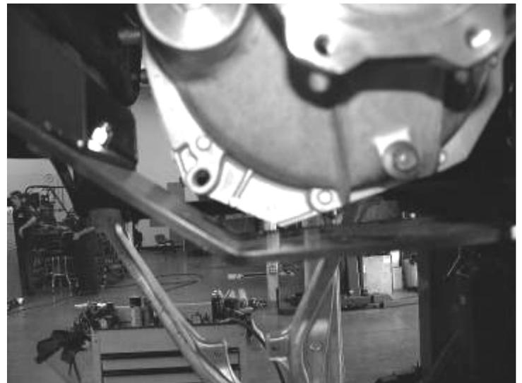
24. Torque the crossmember frame pocket bolts to 125 ft lbs, the lower control arm bolts to 110 ft lbs, the 1/2" skid plate hardware to 75 ft lbs, and the 7/16" to 50 ft lbs.
