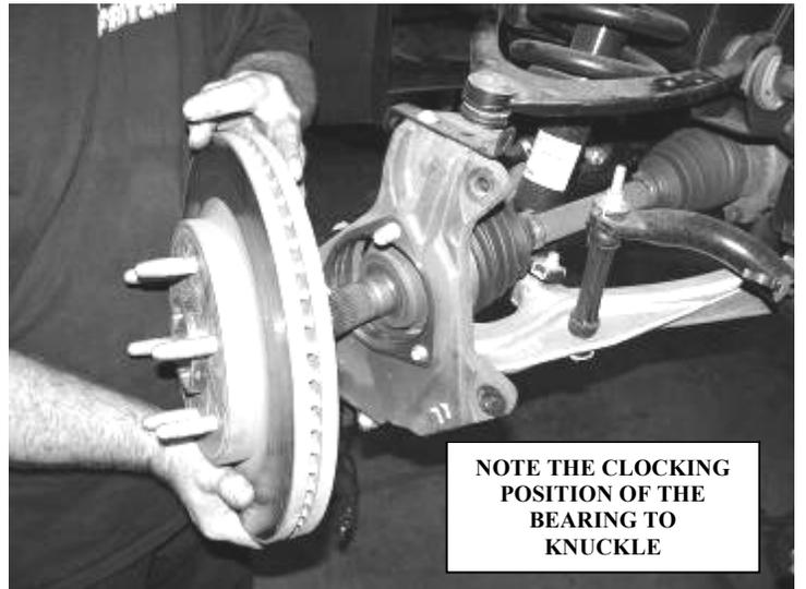
5. Remove the upper and lower ball joint nuts. Disconnect the upper and lower ball joints from the steering knuckle by striking the knuckle with a large hammer next to each ball joint on the knuckle to dislodge the ball joints. Use care not to hit the ball joints when removing. Save nuts and discard knuckle. SEE PHOTO BELOW
