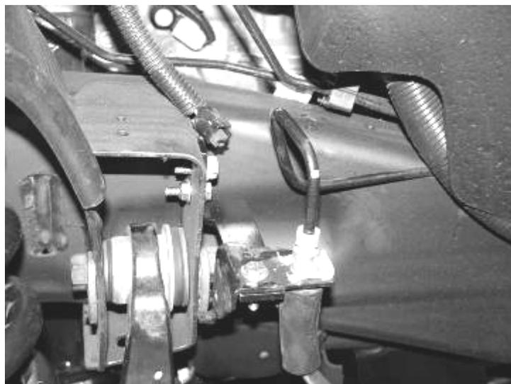
38. Re-route the brake hose and the ABS Line to the steering knuckle using the adel clamp to the back of the steering knuckle and attach with 1/4" x 3/4" bolt and washer. Torque to 10 ft LBS. Route the ABS line next to the brake hose. Re-connect the ABS line to the harness in the wheel well. Using provided plastic tyraps secure line to the hose and away from the tire and wheel. SEE PHOTO BELOW
