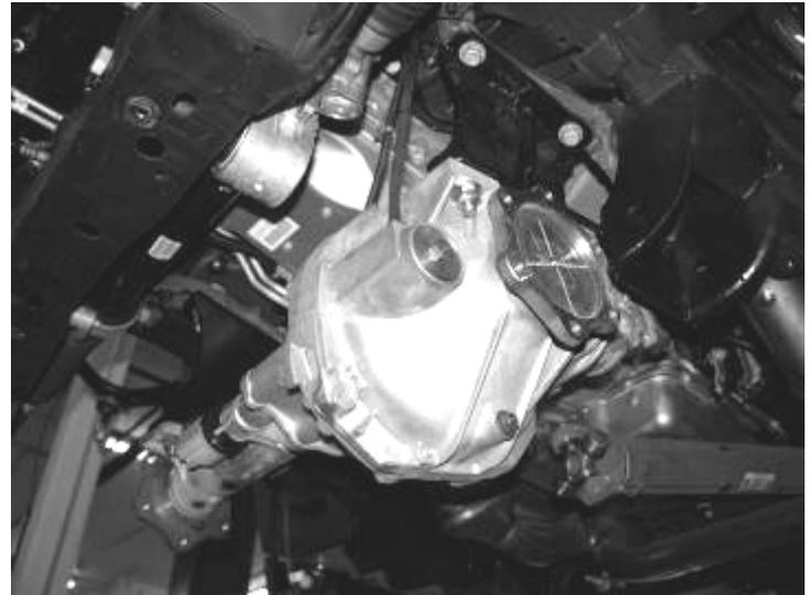
20. Locate and install FT20283 rear crossmember into the factory lower control arm pockets using the stock hardware and leave loose at this time. **(CHECK THE CLEARANCE OF THE DIFF TO CROSSMEMBER WHERE IT WAS SANDED DOWN IN STEP #18 FOR ADAQUATE CLEARANCE TO THE FRAME AND CROSSMEMBER ) SEE PHOTO ON NEXT PAGE.**
