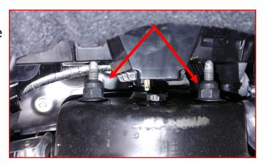
Remove upper control arm bolts located inside strut tower. Remove upper control arm from the vehicle at this time.
