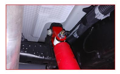
Remove factory bolt that attaches the rear bump stop to frame and discard the bolt.
