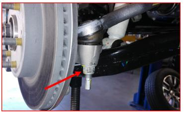
Install the ABS sensor harness and brakeline bracket to the knuckle.
