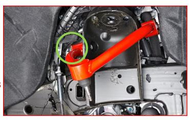
With the upper control arm bolts in place, install the supplied laser cut washers, the supplied M14 washers and nuts.
