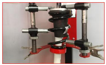
Install factory strut hardware on top hat studs. Mark studs at top of nuts.
