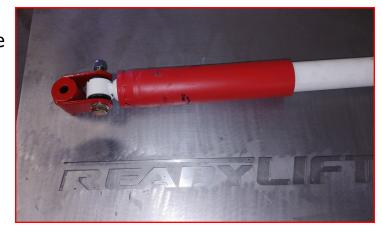
Install the ReadyLIFT shock extension to the frame using factory hardware
