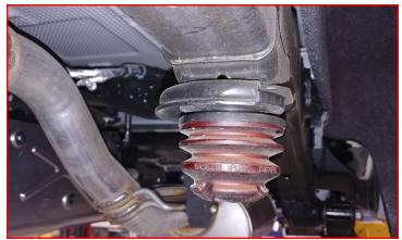
Install rear bump stop extension between frame rail and jounce stop using supplied M10 Bolts and washers. Tighten and torque to 35 ft-lbs.
