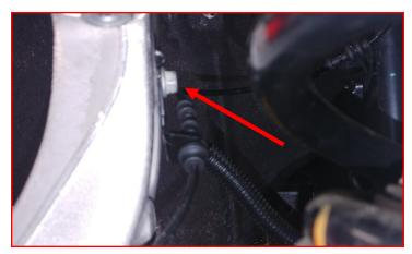
Install the ABS bracket to the Upper Control Arm using supplied 1/4" nut and washer.
