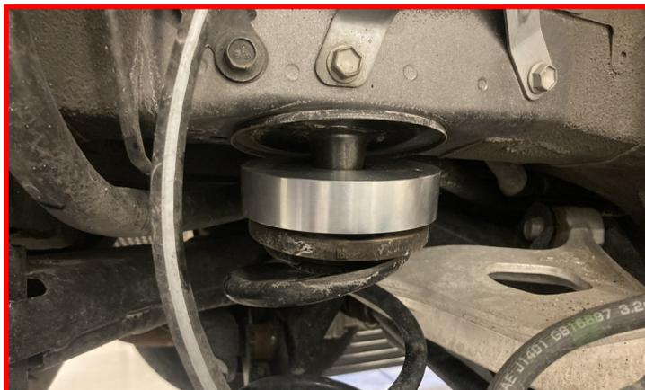
Raise the jack to seat the spacer and spring assembly properly. Make sure to bring the lower control arm into position with the knuckle while raising the jack.
