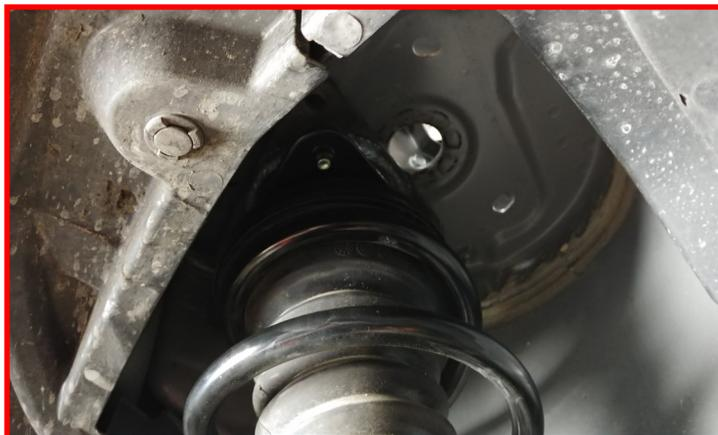
Install the **provided strut spacer** onto the strut mount using the **factory hardware**. This is a tight fit to get the strut spacer and bolts into place. Use of a pry bar may be needed for placement of the strut spacer. The top hat can be rotated to access the bolts. Once all have been started, tighten all down.
