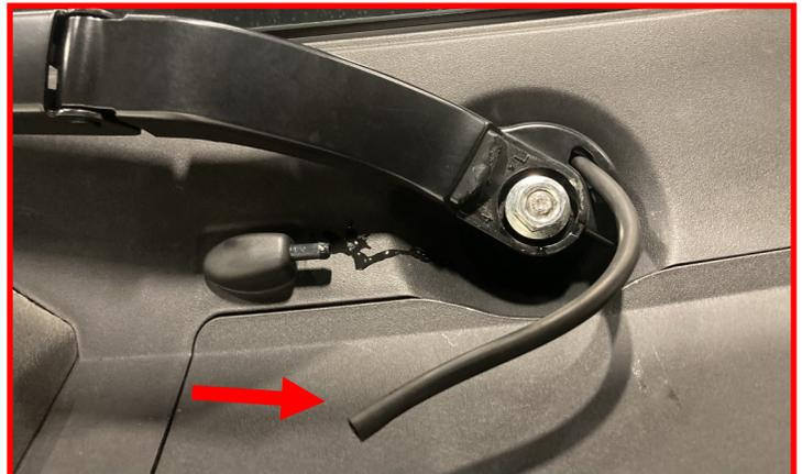
Remove the **factory mounting nut**. Mark the windshield wiper location against the shaft for reinstallation. Gently lift up on the wiper arm while slightly twisting. The arm should pop off the shaft.
