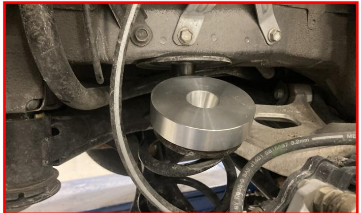
Once complete, position the spring spacer into the factory spring locator.
