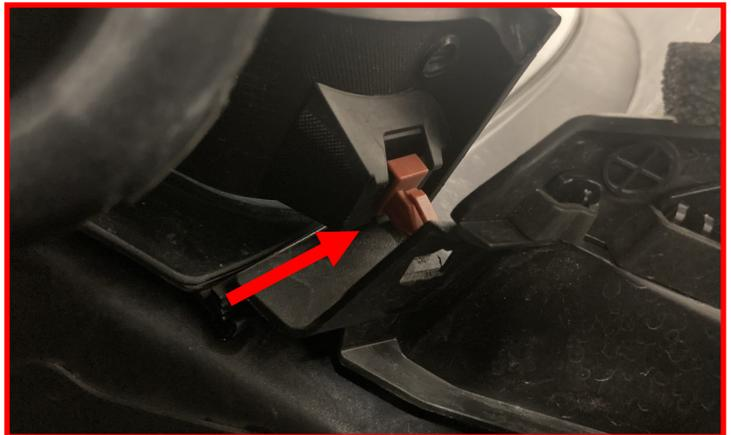
Locate the **x7 plastic clips** holding the cowl to the body. Remove all the clips and set aside. Gently lift up on cowl from the engine bay side, while lifting pull towards the front of the vehicle to disengage from the windshield. Once disengaged from the windshield, set aside in the engine bay.
