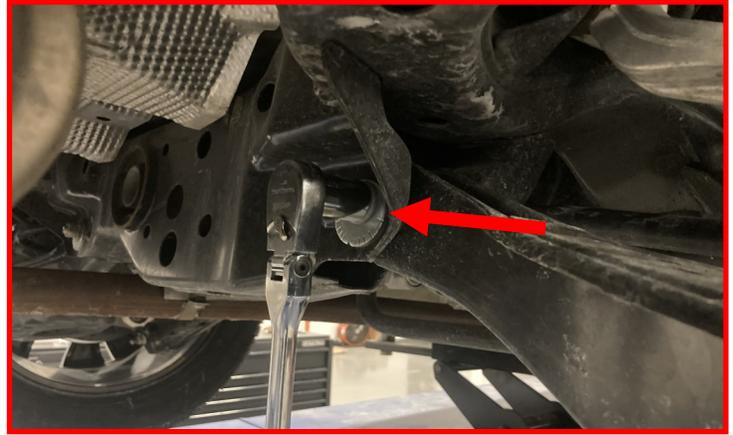
Lower the jack and let the control arm swing down while supporting the spring assembly.
