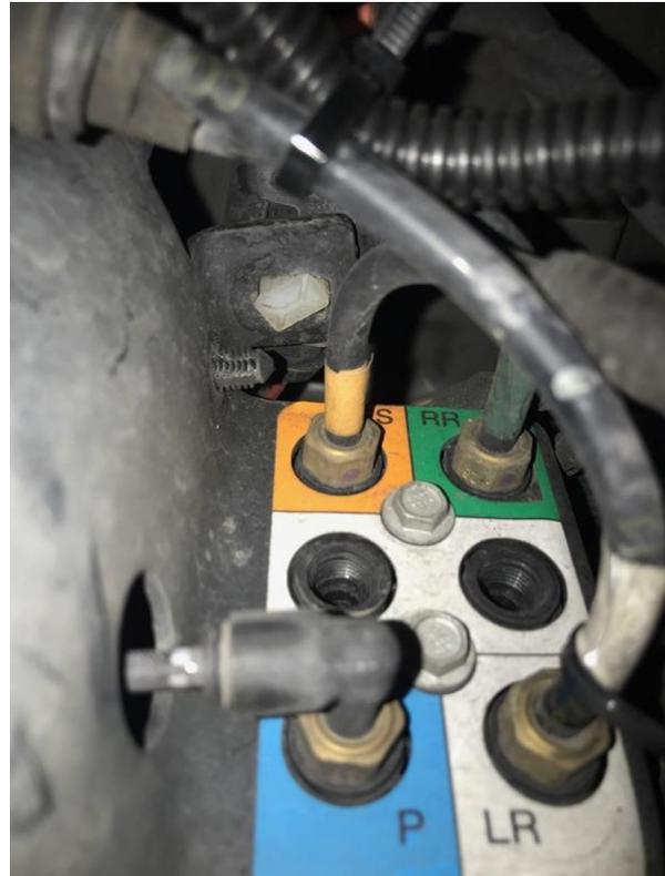
**WARNING!** Make certain the bracket holding the lines to the diff are disconnected or you'll break the brake and air lines.
