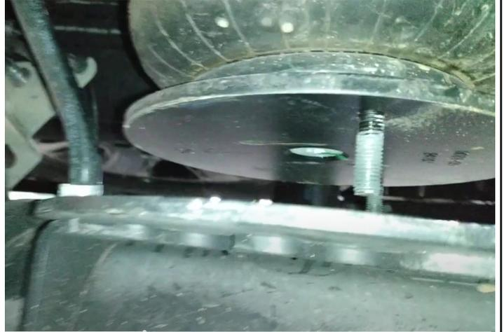
Remove Hex bolt from bottom of air bag to remove lower plate.
