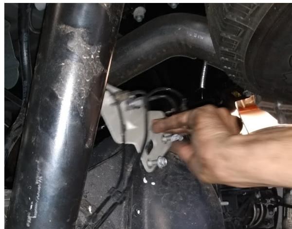
Drop the axle remove the 2 bolts from the bags, lift the airbags
