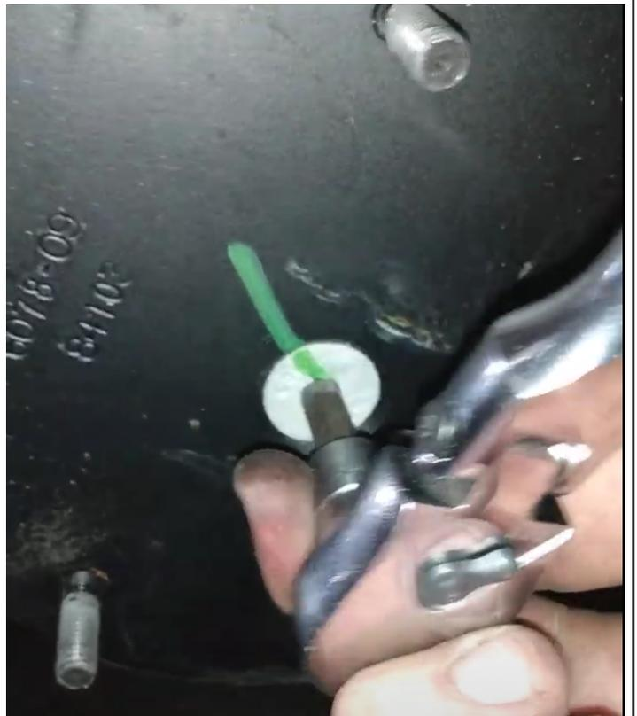
Install Traxda part with supplied 12mmx30x1.75 bolt and use lock washer and plain washer.
