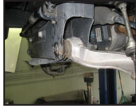
28. Re-install the tie rod ends on each side of the vehicle back into the steering knuckles. Torque to 80 ft lbs.
