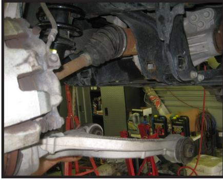
18. Working on the driver side, remove the (3) nuts holding the strut to its upper mounting location and remove the strut from the vehicle. Repeat on passenger side.
