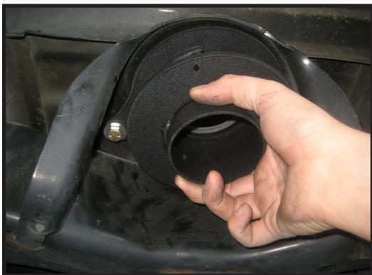
45. Re-install the rear coil springs making sure the OE rubber isolator is between the coil spring and the new coil spring spacer.
