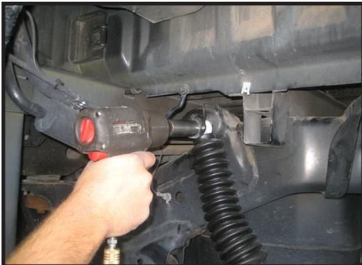
40. Working on the driver side, remove the bolt that holds the brake line bracket to the frame. This is done to gain slack in the brakeline during the install process, save the OE bolt. Repeat on the passenger side.
