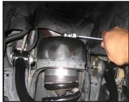
36. Using the provided zip ties, tie the ABS brake wire harness to the upper control arm so that it does not interfere with the bump stop.
