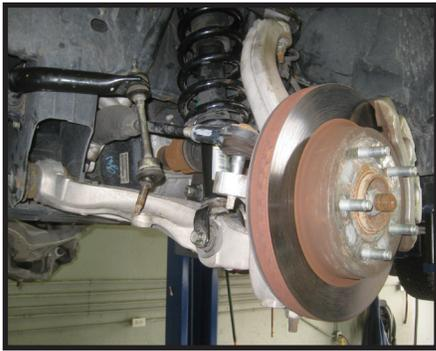
4. Working on the driver side, remove the lower strut mounting bolt and nut, repeat on passenger side.
