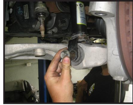
27. Move back the the lower control arm bolts that were removed in step 17 and re-install. Torque to 105 ft lbs.
