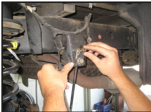
48. Re-install the sway bar endlink upper mounting hardware. Torque to 40 ft lbs.
