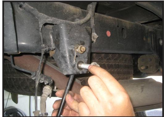
42. Remove the hardware that is attaching the rear Track bar to the axle bracket, save hardware for later installation.
