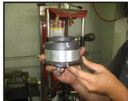
24. Using the wall mounted strut compressor, re-install the strut top plate, preload spacer, and rubber isolator back onto the coil and shock. Secure using the OE hardware and torque to 40 ft lbs.
