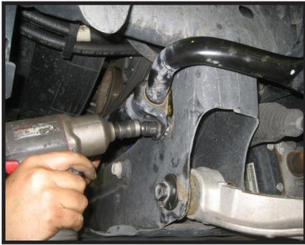
31. Locate (2) 54060-08 sway bar drop brackets, also locate (4) 7/16" x 1 1/2" bolts, (4) 3/8" flat washers, and (4) 7/16" unitorque nuts from hardware bag 34105NB. Install the 7/16" bolts into the sway bar drop brackets as shown in the picture below.
