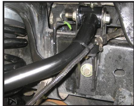
37. Tuff Country highly recommends at this time to grease the (4) grease fittings on each eylet of the upper control arms, this will prevent squeaking and premature wear and tear of the bushings.
