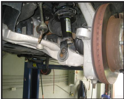
5. Now is a good time to have a jack set up under the lower control arms to support the suspension from dropping suddenly.
