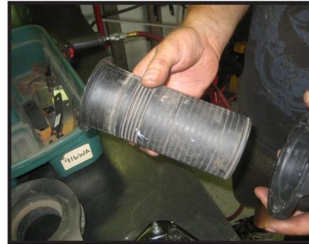
22. Locate the new 34105-04 front strut pre-load spacer and install it into the top strut plate
