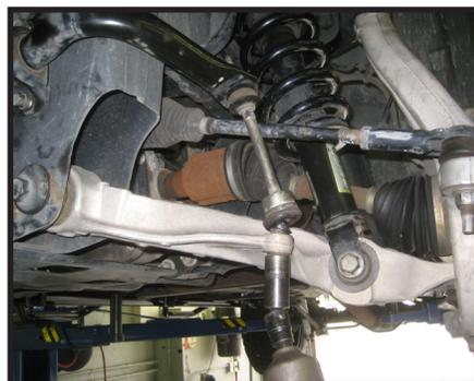
3. Working on the driver side, detach the tie rod end from the steering knuckle by removing the nut, and breaking the taper using a hammer or suitable tie rod removal tool. Repeat on passenger side. **Special note: be extra careful to not damage the tie rod end rubber boot or threads while performing this step.**
