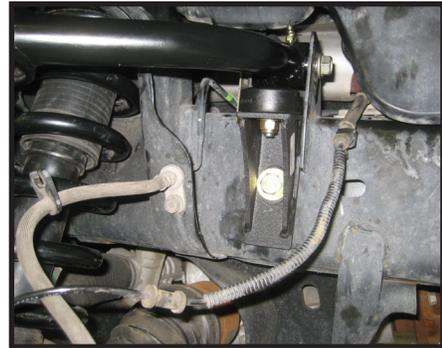
17. Working on the driver side Lower control arm, remove the 2 bolts connecting it to the frame of the vehicle, carefully pry the control arm out of its pockets and let it hang in the air. Repeat on passenger side.
