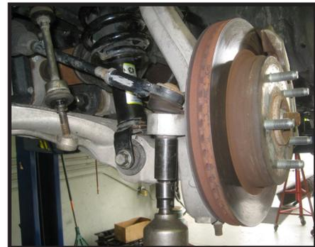
29. Move back to the lower strut mounting hardware and torque to 95 ftlbs.
