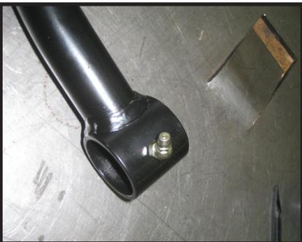
10. Locate (8) TC-002 control arm bushings, and (4) S10254 crush sleeves from hardware bag 34105NB1. Install the bushings and sleeves into each control arm. **Special note: Make sure to use a fair amount of lithium or moly base grease before installing the new bushings and sleeves into the control arms. This will increase the life of the bushing as well as help prevent squeaking.**
