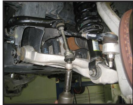
35. Move back to the 3/8" upper strut hardware from step #26 and torque to 28 ft lbs.
