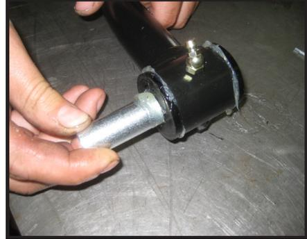
11. Working on the driver side, Install the new upper control arm into the vehicle using the OE hardware. Torque to 75 ft lbs. Repeat on passenger side.
