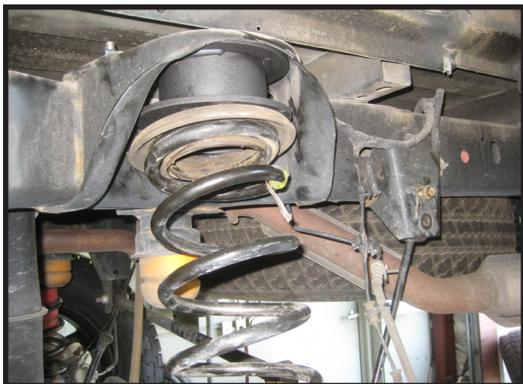
46. Re-install the rear track bar back into its OE mounting bracket using the OE hardware. Torque to 85 ft lbs
