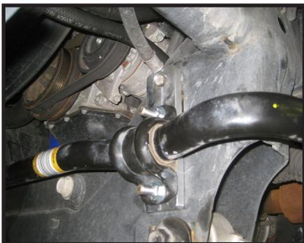
34. Install Sway bar endlinks back into the lower control arm and secure using the OE nut. Torque to 45 ft lbs.
