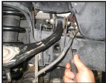
8. Working on the driver side, remove the 2 bolts that are holding the upper control arm on the vehicle, then remove the control arm from the vehicle. Repeat on passenger side.
