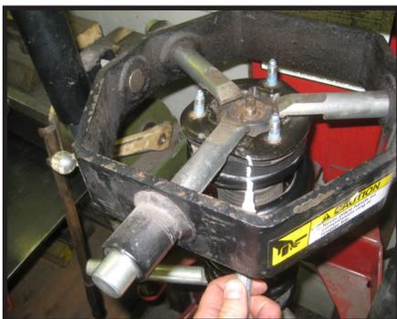
20. Remove the hardware that is attaching the shock to the upper strut plate, then relieve all of the pressure off of the strut so that the top plate can be removed.
