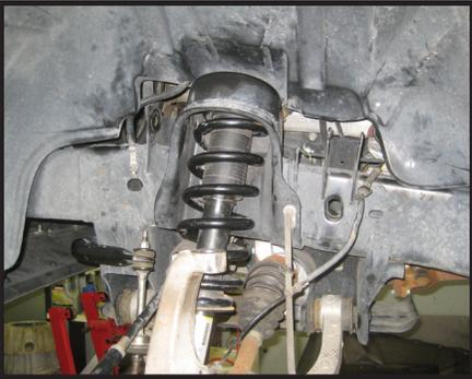
9. Locate the new upper control arms, also locate the (4) grease fittings from hardware bag 34105NB1. Install the grease fittings into each eyelet of the control arms so that they are facing towards the outside of the vehicle. **Special note: Be extra careful not to over tighten these small brass grease fittings.**
