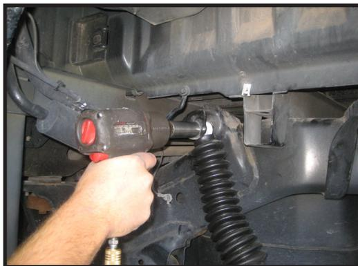
51. Re-install the rear inner fender liners using the OE bolts.
