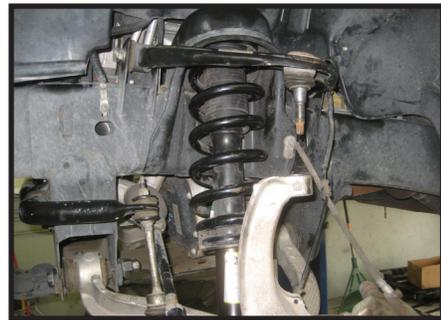
7. Working on the driver side, remove the ABS line clip that is connected to the upper control arm mount. Repeat on passenger side.
