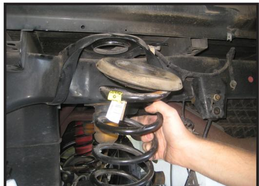
44. Locate (2) 34105-03 rear coil spacers, also locate (2) 7/16" x 1 1/2" bolts, (2) 3/8" flat washers, and (2) 7/16" uni-torque nuts from hardware bag 34105NB. Working on the driver side, install the coil spacer into the upper mounting point of the frame and secure it using the new 7/16" hardware. Torque to 42 ft lbs. Repeat on passenger side.
