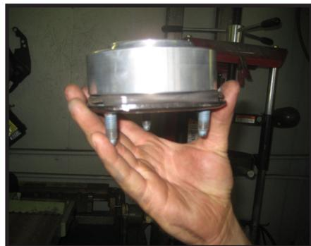
23. Install the OE rubber isolator onto the newly installed strut pre-load spacer and make sure to line your marks up.
