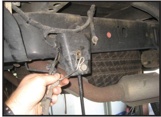
41. Working on the driver side, remove the hardware that attaches the swaybar end link to the frame mount, save the hardware and repeat on passenger side.
