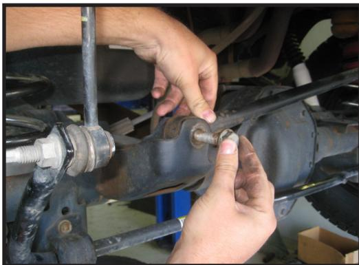
47. Re-install the brakeline bracket mounting hardware. torque to 8 ft lbs.
