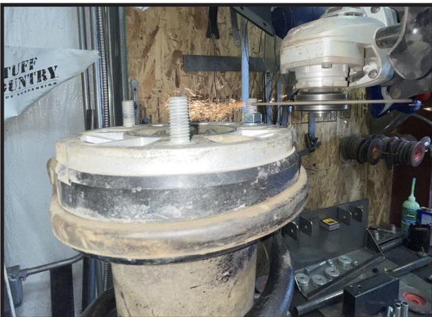
27. Remove the flange nuts and this will clear any rough edges from cutting the studs
