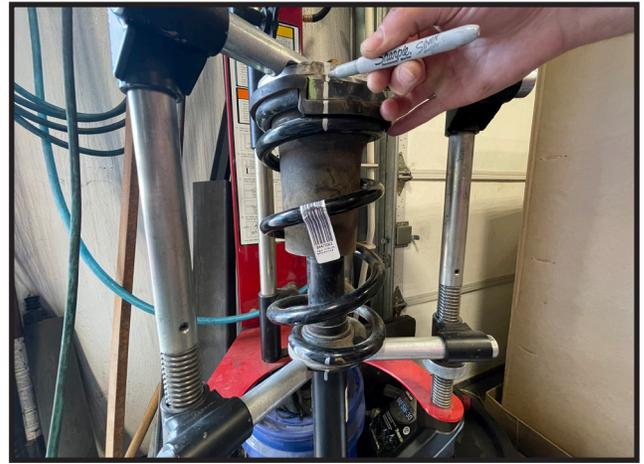
20. Relieve the pressure from the strut top hat, remove the OE nut, top hat, and coil spring. Save hardware for later re-installation.
