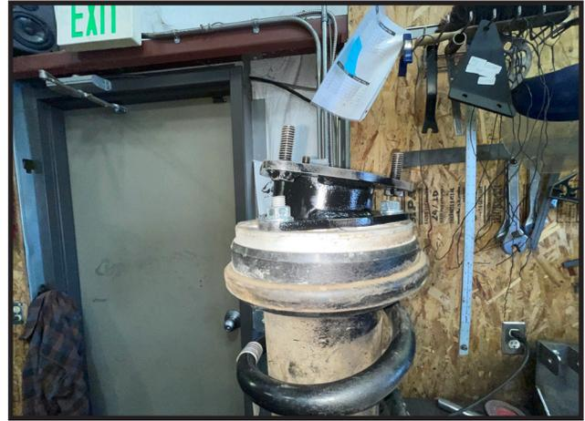
29. While the strut is still on the bench, Remove the (2) OE clip nuts from the bottom mount of the shock and discard.
