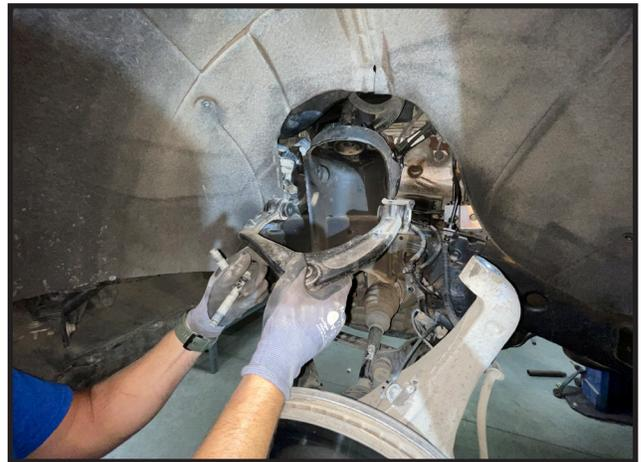
13. Locate the new Driver side upper control arm, also locate (4) Polyurethane bushings, (2) crush sleeves, and (2) grease fittings. Using a polyurethane compatible grease, apply a healthy amount on the bushings and crush sleeves, then install into the new upper control arms.
