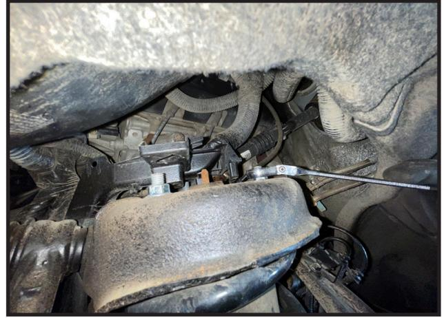
7. Once upper hardware is removed, carefully remove the strut from the vehicle and set aside
