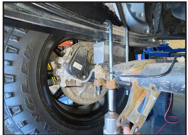
7. Repeat on the passenger side and once both blocks and u-bolts are installed **torque the u-bolts to 110 ft lbs.**
