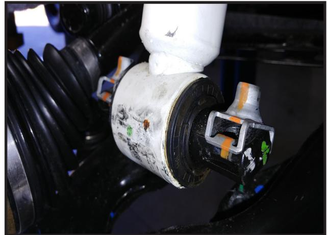
30. Locate (3) 3/8" flange nuts, Install the strut assembly back into the vehicle and loosely start only 1 of the 3/8" flange nuts on the outer most upper stud.
