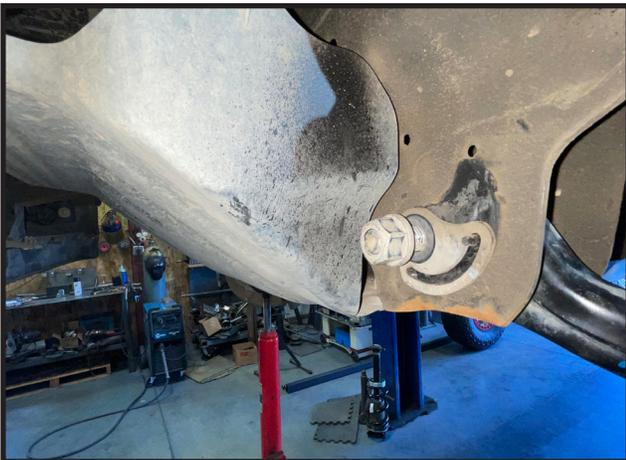
34. Move back to the strut lower mounting hardware that were installed on STEP #31 and **Torque to 42 ft lbs.**
