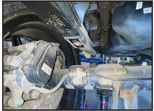
5. Install the new lift block between the bottom of the leaf spring and the perch on the axle making sure alignment pin and hole are lined up.
