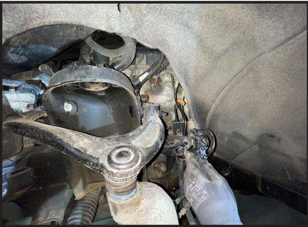
10. Using a floor jack or suitable tool, support the lower control arm so that the front suspension cannot drop down.
