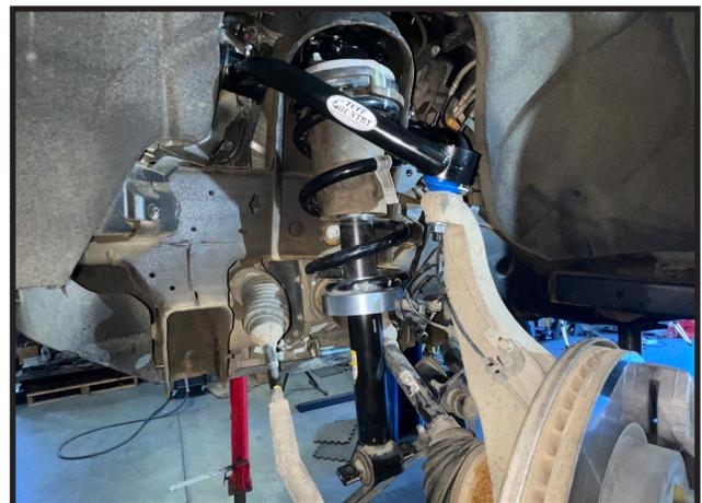
31. Locate (2) 10mm x 60mm bolts, (4) 10mm flat washers, and (2) 10mm unitorque nuts. Carefully raise up the lower control arm so that the lower strut mounting points are lined up and install the new 10mm hardware with the bolt heads facing up. **Do not tighten at this time.**
