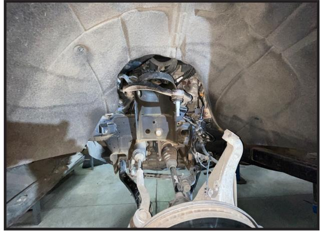
12. Remove the 2 bolts and hardware that attach the upper control arm to the vehicle, and remove the OE upper control arm.
