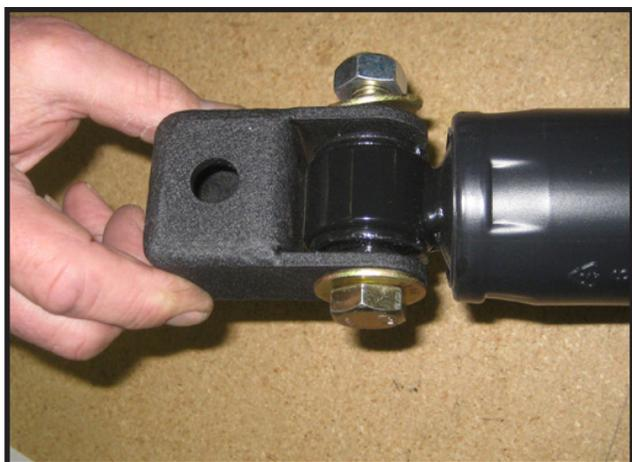
10. Re-install shocks using the OE hardware.
