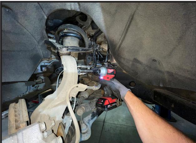
4. Remove the lower control arm mounting bolts and hardware and save.
