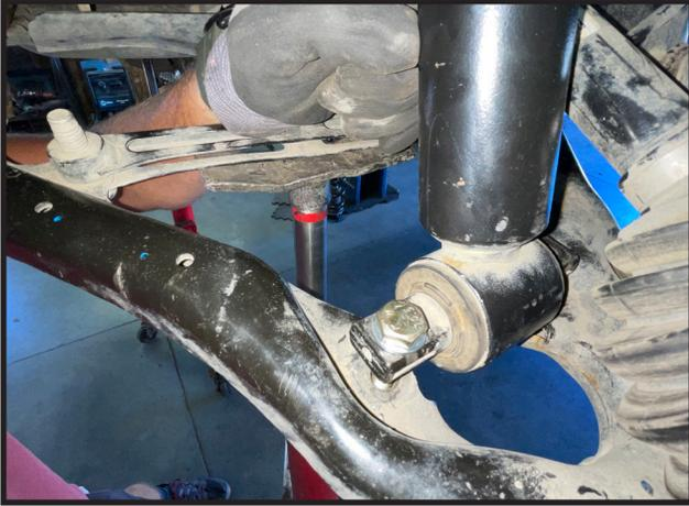
32. This step can be tricky, but you need to continue raising up on the lower control arm so that the eyelets go back into the mounting pockets.
