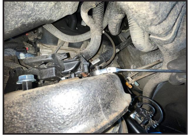
36. Locate (1) 1/4" unitorque nut, and (1) 1/4" flat washer, and install the ABS wire harness mount onto the welded stud of the new upper control arm.
