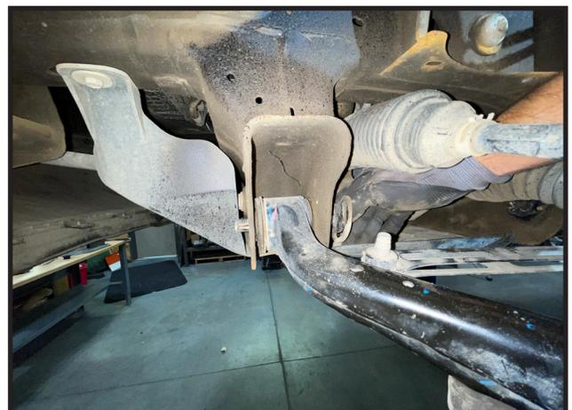
9. Remove the ABS wire harness mounting bracket from the upper control arm and pull aside.
