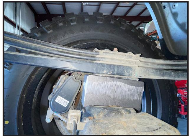
6. Secure using the new u-bolts and hardware. **Snug the u-bolts at this time but do not fully torque yet.**
