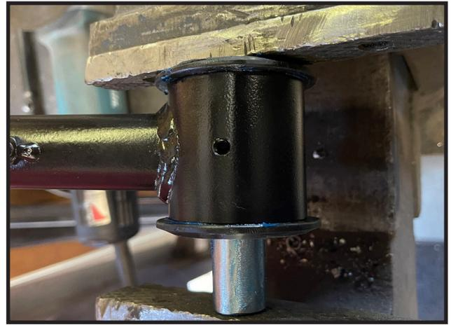
14. Carefully install the grease fittings into the threaded holes of the upper control arms. **Be careful to not over tighten these as they are made of brass and can easily strip out.**
