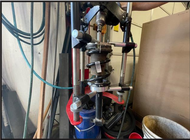
26. Take the strut assembly out of the compressing tool and take it to the bench. Install the new supplied 10mm flange nuts and thread them all the way down on the 3 studs on top of the strut. Using a cutting tool, cut 1/4" (roughly 3-4 threads) off of the top of the **2 outer** OE studs to make them short enough to clear the new strut spacer. Next cut the **1 inner** stud off flush with the top of the flange nut
