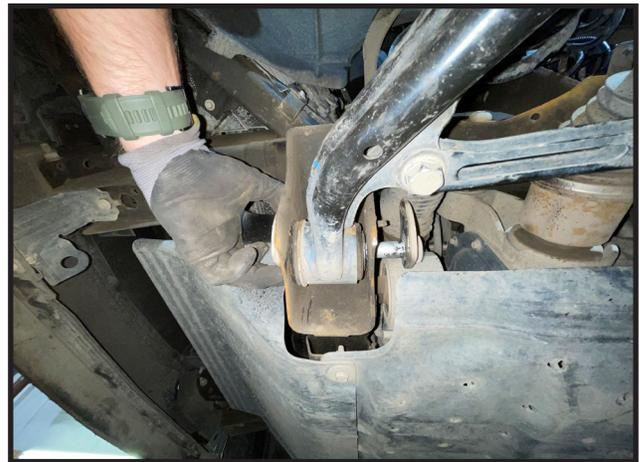
5. Working on the lower strut mount, remove the 2 bolts that attach it to the lower control arm. **Special note: when these bolts are out, be careful that the lower control arm doesn't drop and swing away too fast and damage anything.**
