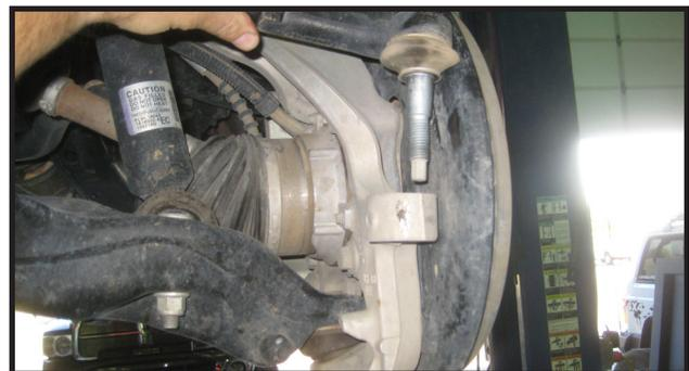
4. Working on the driver side, remove the sway bar endlink from the steering knuckle. Save nut for re-installation.
