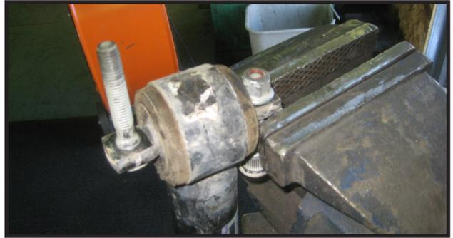
24. With the studs removed from the lower strut mount, you will now be able to re-install the strut assembly back into the vehicle. Locate (3) 3/8" flange nuts. Loosely start the nuts on the upper strut mount so the strut can still be maneuvered around. **Note: It is usually necessary to un-pin the lower control arm from the frame pockets again, to allow enough room to install the strut.**
