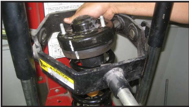
22. Locate a new upper strut spacer part # 22909-01 and install it on the top of the strut using the new M10 serrated flange nuts. **Torque nuts to 35 ft lbs.**
