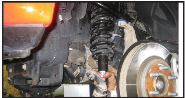
25. Line the lower strut mount up with its mounting holes on the lower control arm and re-install the (2) studs. Use the nuts to tighten and suck the studs back down into the mount.
