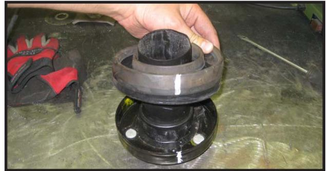
18. Place a clamp on the lower coil spring and mount so tha the shock does not fall to the ground when the nut is removed.
