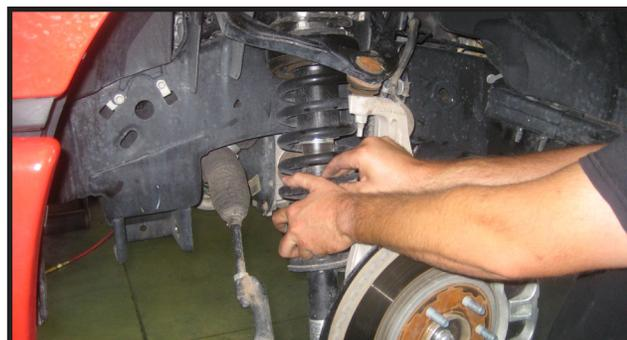
9. Re-attach the lower control arm to the mounting pockets on the frame rail. The bolts only need to be pinned and not tightened, as this is just to hold the lower control arm and steering knuckle up while the new upper control arm is installed.
