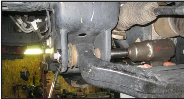
27. Return to the (3) 3/8" nuts on the upper strut mount and tight them down. **torque to 45 ft lbs.**
