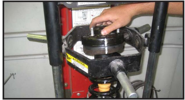
20. Locate the new pre-load spacer. Place the bearing plate on a work bench upside down. Remove the rubber isolator and install the pre-load spacer in its place. Re-install the rubber isolator making sure to line up your marks made earlier.
