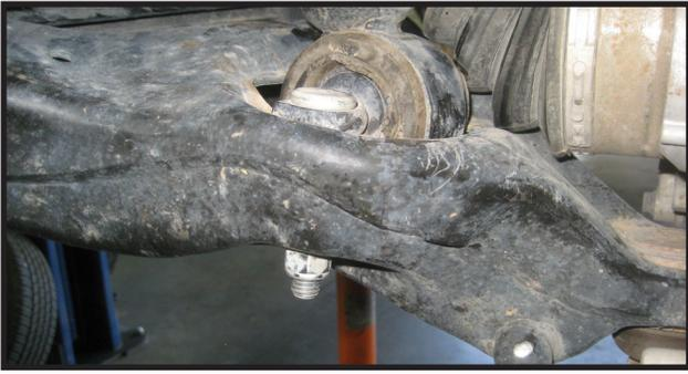
26. If you un-pinned the lower control arm in Step # 24, at this time, re-attach the lower control arm to the frame pocket mounts and secure using the OE hardware. **Torque bolts to 115 ft lbs.**
