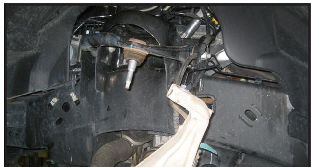
11. Remove the upper control arm from the vehicle, saving the hardware for later re-installation.
