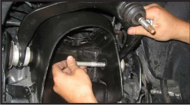
12. Locate the new driver side upper control arm part # 20930-11. Also locate (4) TC-002 bushings, (2) S10236 crush sleeves, and (2) SERT06 grease fittings. Install the bushings and sleeves into the new upper control arm. **Special note: Make sure to use a fair amount of lithium or moly base grease before installing the new bushings and sleeves, this will increase the life of the bushing as well as help prevent squeaking.**
