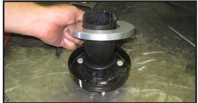
19. Carefully compress the strut until the upper bearing plate can be removed. Remove the nut and hardware and save for later re-installation.
