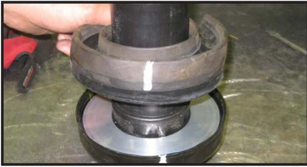
21. Install the modified bearing plate back into the strut using the OE hardware. **Make sure that all the reference lines you scribed earlier line up with each other to make installation much easier.**
