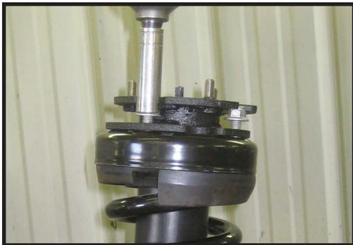
23. Secure the lower strut mount in a bench vise so that the (2) studs can be knocked out with a hammer. Make sure to thread a nut on the studs so that you don't damage the threads
