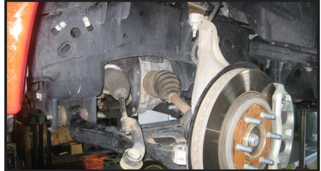
10. Remove the nut from the upper ball joint where it attaches to the steering knuckle. Carefully separate the ball joint from the steering knuckle by striking the knuckle with a hammer.
