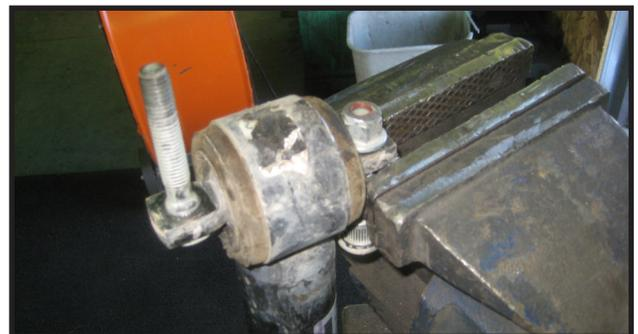
18. With the studs removed from the lower strut mount, you will now be able to re-install the strut assembly back into the vehicle. Locate the OE upper strut mounting hardware and Loosely start the nuts on the upper strut mount so the strut can still be maneuvered around. **Note: It is usually necessary to un-pin the lower control arm from the frame pockets again, to allow enough room to install the strut.**
