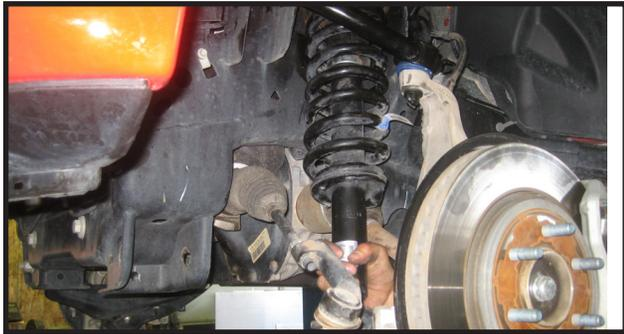
19. Line the lower strut mount up with its mounting holes on the lower control arm and re-install the (2) studs. Use the nuts to tighten and suck the studs back down into the mount.
