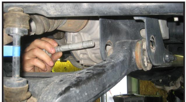
7. At this point, the lower control arm will need to be dropped down away from the lower strut mount. **Be extra careful to not over extend any brakelines or the CV axle while performing this step.**
