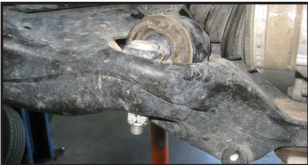
20. If you un-pinned the lower control arm in Step #18, at this time, re-attach the lower control arm to the frame pocket mounts and secure using the OE hardware. **Torque bolts to 115 ft lbs.**
