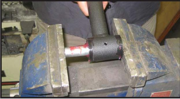
13. Install the new grease fittings into the threaded holes of the eyelets on the upper control arm. **Careful to not over tighten the fittings, they are soft brass and can easily be stripped out.**
