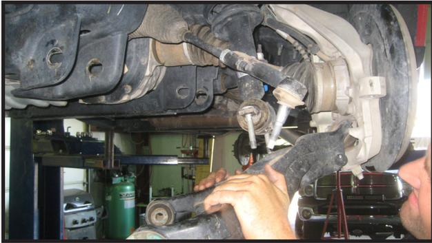
8. Remove the (3) mounting nuts on the upper strut mount and remove the strut from the vehicle. Set strut assembly aside.
