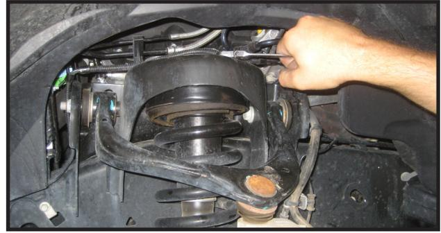
22. Re-install the tie rod end into the steering knuckle and **torque nut to 95 ft lbs.**
