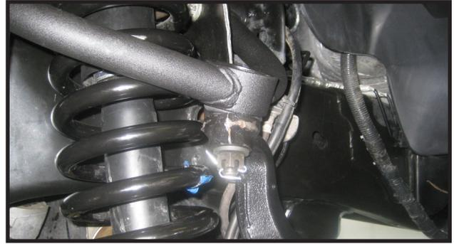
16. At this time it may be necessary to slightly bend the break line mounting bracket that is located on the rear pocket of the upper control arm. This will allow the new upper control arm to fully travel downward.
