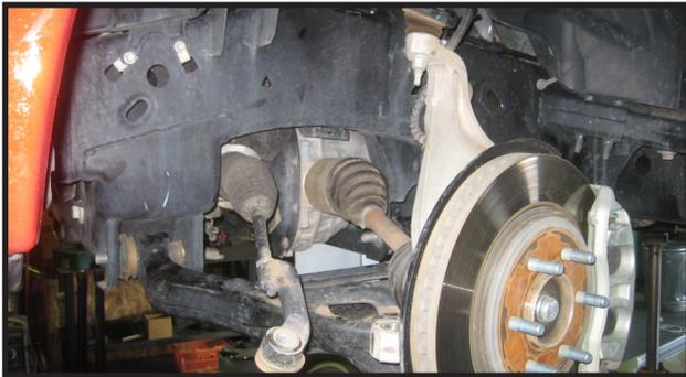
10. Remove the nut from the upper ball joint where it attaches to the steering knuckle. Carefully separate the ball joint from the steering knuckle by striking the knuckle with a hammer.
