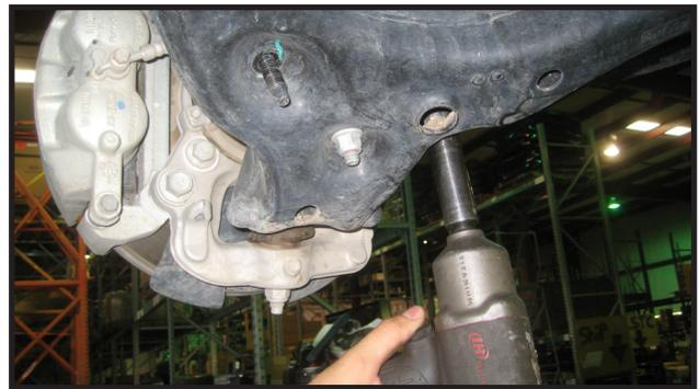
6. Remove the 2 bolts that connect the lower control arm to its pocket mounts on the frame rail.
