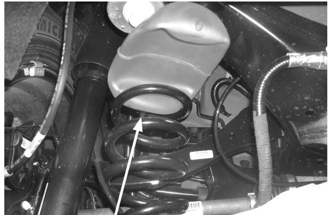
Insert cylinder with stem pointing down
