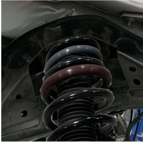
29. Reattach the upper strut bolts with a 15mm wrench and torque to 41 lb.ft.
