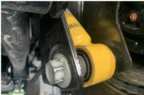
12. Remove upper strut bolts with a 15mm wrench.
