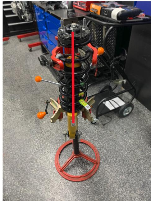
15. Compress the spring until tension is relieved from the strut.
