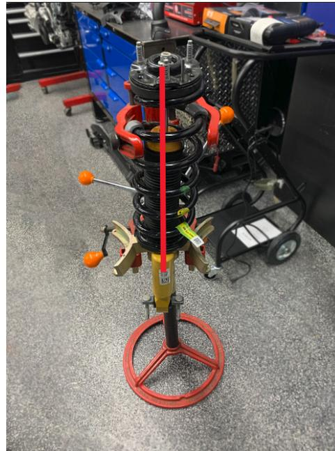
16. Compress the spring until tension is relieved from the strut.
