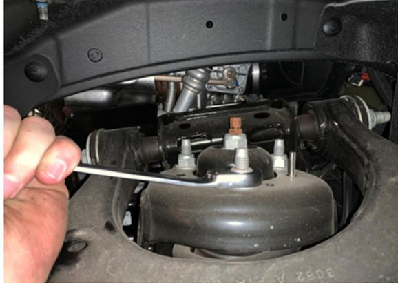
30. Attach the lower strut mount to the lower control arm using the supplied bolts and Nylock nuts. Torque the supplied nuts to 80ft-lbs.
