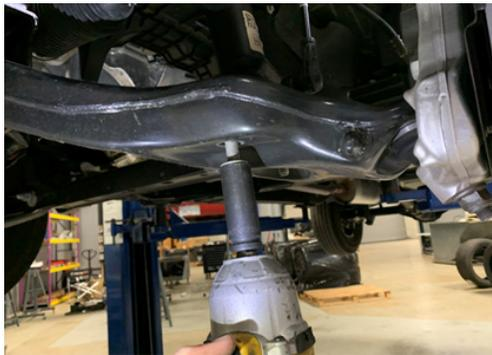
31. Reattach the lower control arm to the frame using the OE alignment hardware. Do not tighten or torque until your vehicle is back on the ground.
