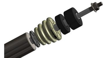
26. With the OE spring still compressed, slide the strut back into the spring and put the top mount back on.
