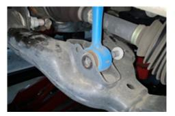
13. Using an oil-based paint pen, mark the alignment of the camber and caster adjustment bolts securing the lower control arm to the frame. When reinstalling the control arms later, this will help keep the alignment close to proper settings.
