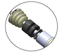
26. With the OE spring still compressed, slide the strut back into the spring and put the top mount back on.
