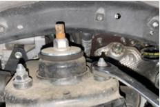
16. Remove the strut from the vehicle. Some additional adjusting of the spindle's location may be necessary to drop the strut down. Be careful not to separate the joints of the axle by pulling on the spindle too much.
