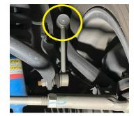
10. Disconnect the tie rod by removing the cotter pin and Castle nut. Strike the designated area carefully on the spindle to dislodge the tie rod.
