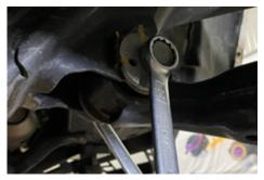
15. With the lower control arm swung out of the way, the strut should be held only by the three nuts on the top mount. While holding the strut up to avoid dropping it, loosen and remove the top three nuts using a 14mm wrench.
