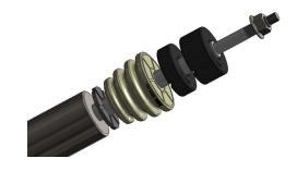
23. Confirm the vent desk is located on the strut, under the dust boot. If for any reason your vent disk is not present, please call our technical support staff before proceeding, as driving on the strut without it could cause the shock to fail.
