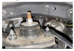
16. Remove the strut from the vehicle. Some additional adjusting of the spindle's location may be necessary to drop the strut down. Be careful not to separate the joints of the axle by pulling on the spindle too much.
