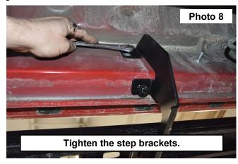
9. Tighten the hardware using a 10mm wrench on each of the (4) mounting brackets. See Photo 9.
