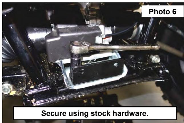
6. Install the upper bracket over the upper holes and secure with the stock hardware and supplied hardware. Tighten supplied hardware using a 16mm socket/wrench. See Photo 7 and Photo 8.
