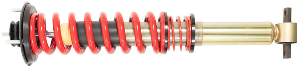
15. Depending on your desired ride height, remove the Belltech top mount and main spring and using the tables below as reference, slide the required packers off the strut rod.
