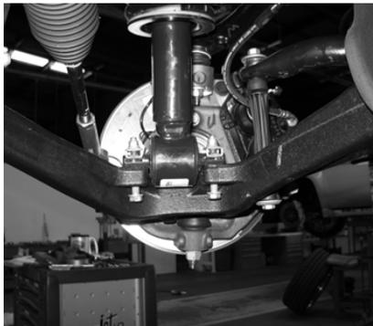
12. Remove the mount nuts from the end links. Remove the end links completely. Doing so allows the lower control arms to droop further and ease the strut removal.
