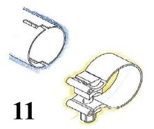
WARNING: Use extreme caution during installation. Torque all fasteners according to manufacturer's torque values and tightening sequence. <u>DO NOT</u> use air impact tools to tighten fasteners on Borla Performance Exhaust Systems. Use of such tools may result in bent flanges or gasket contact areas leading to exhaust leaks.
