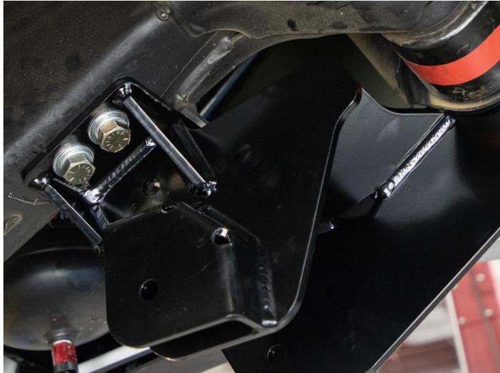
10. Locate two (2) **8460** Cognito Traction Bar Shackles and **HP9214**. Find four (4) **6715** shackle bushings and two (2) **5036** crush sleeves from within the hardware pack. Install two (2) bushings and one (1) crush sleeve per shackle, see Figures 7 and 8.
