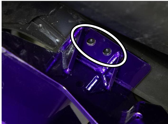
7. Either loosen the forward leaf spring mounting bolt and swing the frame mount bracket away from the frame or use the frame mount bracket as a drill template, and drill through the bottom side of the frame using a 1/2" drill bit, see Figure 4.
