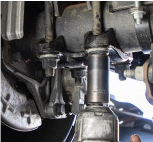
*Figure 12: Leaf Spring Axle Bracket Installation*
