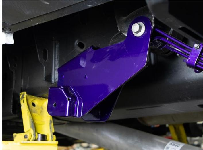
6. Use a center punch to mark the location of the mounting holes onto the vehicles frame, see Figure 3.
