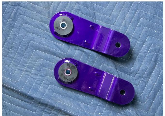
11. Locate **HP9205** and install the assembled shackles to the frame mount bracket using two (2) 1/2"-13 x 2.25" bolts, two (2) 1/2" flat washers, and 1/2"-13 lock nuts, see Figure 9.
