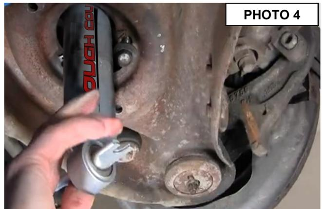
9. Now that the stock shock is removed, take your RC shock and feed it through lower arm. **See Photo 4**
