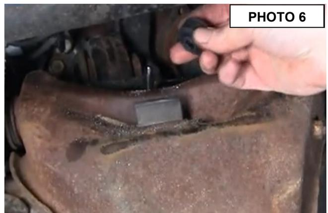
11. Cut winding holding shock compressed and guide stem into hole in the upper coil hat.
