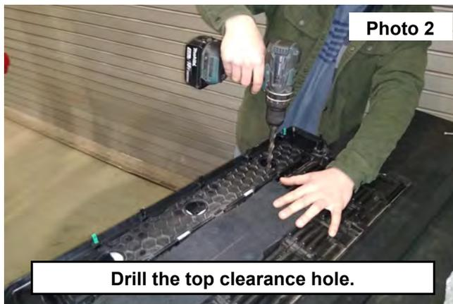
3. Locate the 2 dimples in the bottom of the tail gate trim panel. If needed hold the new table frame up to the tailgate and make a note of where the mounting holes are in the table frame that line up with the threaded holes in the tailgate. Drill the clearance hole using a 1/2" drill bit. **See Photo 3.**
