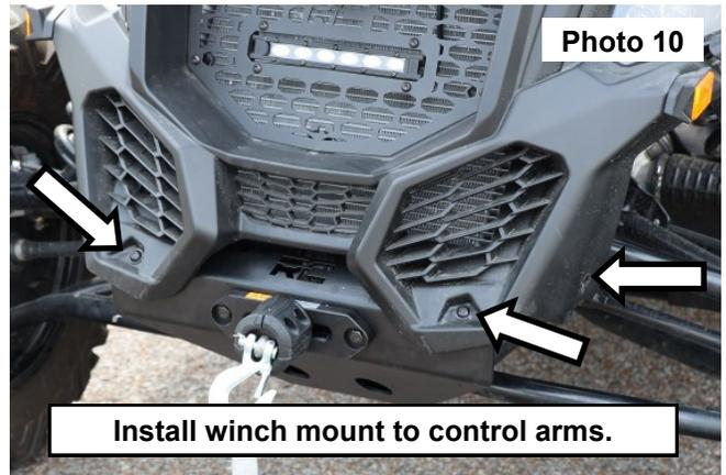
10. Wire the winch to the UTV according to the supplied instructions in the winch kit.
