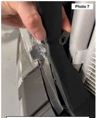
Place the clip over the drilled hole.
