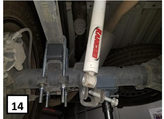
f) Remove the factory U-bolts by evenly undoing the nuts using a 21mm socket, then remove the factory blocks. Slowly lower the axle using the floor jack to allow for the new 3" block to be installed. **(PHOTO 15)**
