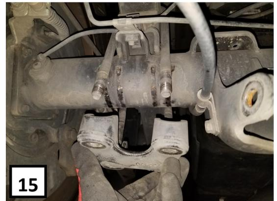
g) Install the block on the factory spring pad with the flat part of the block on the spring and the tapered end towards the front. Jack up the axle to meet the springs, making sure to align the center pin.
