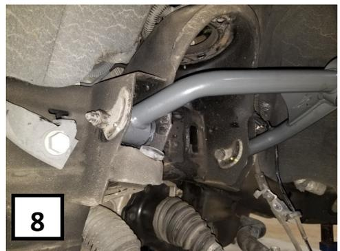
**FIGURE:1 CONTROL ARM BUSHING ASSEMBLY**
