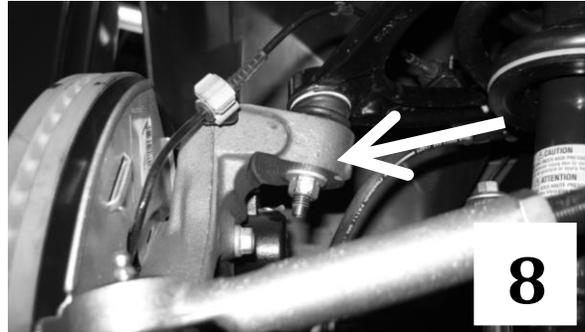
5b. Re-install the sway bar end links to 18ft-lbs.
