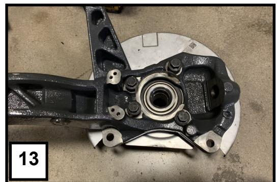
19. Remove the hub and brake backing plate from the factory spindle using an 18mm socket. Install on the Lift Spindle. **(PHOTO 13)**
