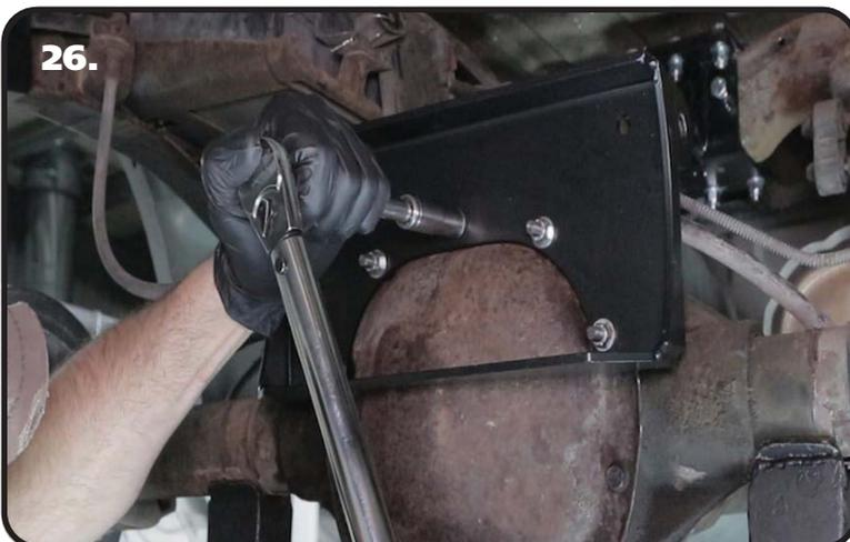
**26.** Line the 5 holes in the axle bracket with the 5 studs that were just installed in the axle housing. Using the Hardware Bag "Upper Wishbone Differential Mount", install a 5/16" flat washer, followed by a 5/16"-18 Nylok Nut on each of the (5) studs. Torque the nuts to 25 ftlbs.
