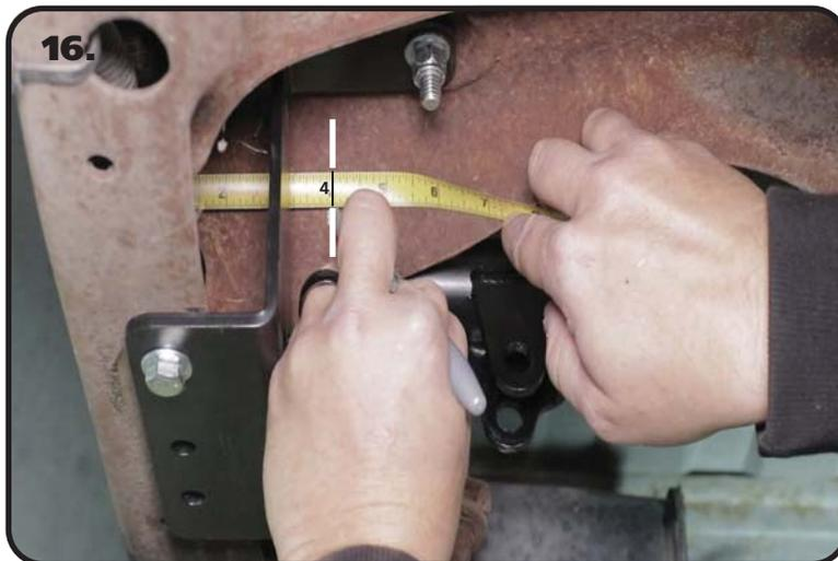
**16.** The NEW crossmember has a tab that rests against the top of the OEM shock crossmember. A hole will need to be drilled from the bottom side. The next 2 steps show you how to mark the hole location from the bottom. Measure over 4" from the inside of the frame rail and put a couple marks above and below the tape measure tape.
