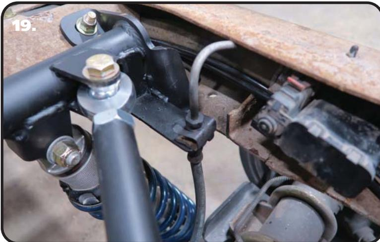
**19.** Attach the brake line to the brake line bracket on the driver side of the upper crossmember. The brake line will slip in the opening of the bracket. Reinstall the clip that was removed earlier.
