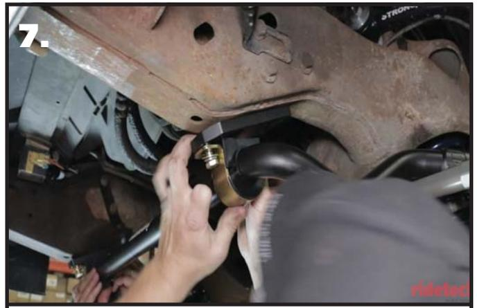
**7.** Slide the SwayBar into position on the S10 with the SwayBar arms above the tie rods. Install a 3/8" Lock Washer & 3/8" Flat Washer on the 3/8"x 3/4" Hex Bolts. Do **NOT** Complete tighten the Hardware, it will be left partially loose until the End Links are installed.
