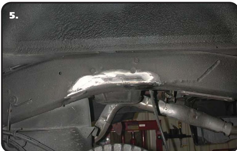
5. Grind the frame smooth after removing the bumpstop bracket. We recommend painting the area to prevent future rust.
