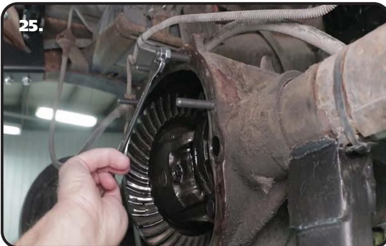
**25.** Thread the stud into one of the 5 threaded holes in the axle housing. Torque the stud to 25 ftlbs. Use 2 wrenches to unlock the nuts from each other and remove them from the stud. Repeat the process on the remaining 4 studs.
