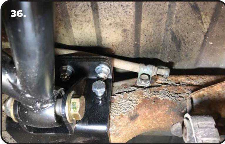
**36.** Image 36 illustrates where we moved the differential vent that was on top of the crossmember. It will bolt in the hole that the emissions modules was bolt into using the OEM hardware.
