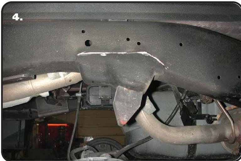
4. Remove the OEM bumpstop and bracket. A die grinder with a cutoff wheel works well for this. We use the cutoff wheel to cut the weld, taking care to not cut into the frame.
