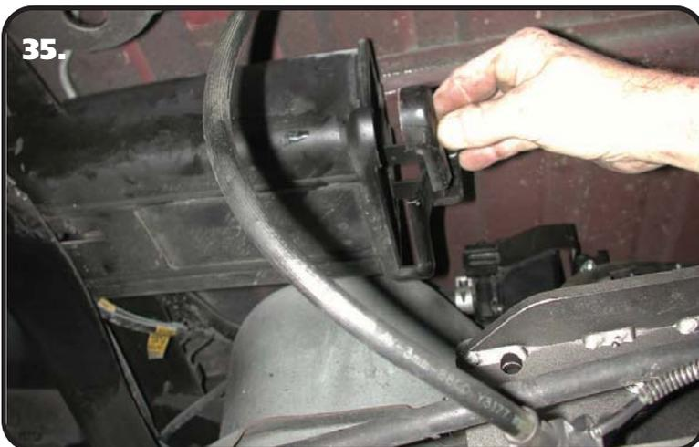
**35.** This particular truck had the emissions canister mounted right behind the gas tank. We had to trim the rear corner off for clearance of the new lowered suspension.
