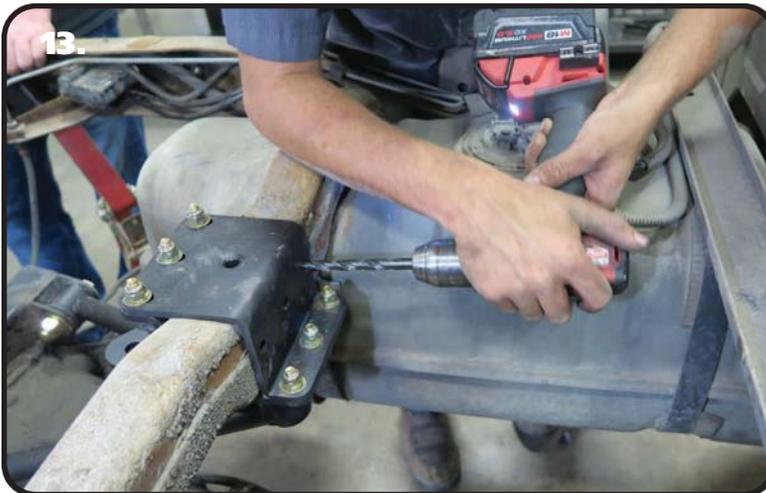
**13.** The wishbone mount has (3) holes in the front and rear that need to be drilled with a 3/8" drill bit. Use the wishbone mount as a template to drill the front and rear holes. Drill the (3) front holes and (3) rear holes from their respective sides.
