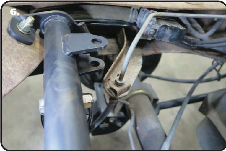
Steps 6-8 cover removing the rear brake line bracket from the frame rail. You can disconnect the metal line from the rubber line, but you will need to bleed the rear brakes. We are going to illustrate how to remove the bracket without opening the rear brake line.
