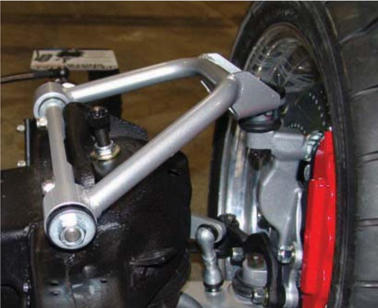
1. Fasten the upper arm to the frame using the OEM hardware with the supplied Washer under the nut. Reinstall the current alignment shims, but **vehicle must be realigned**.
