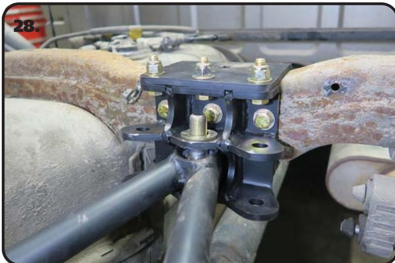
**28.** Insert a narrow R-Joint spacer (.620") into each side of the front R-joint of the wishbone. Using the Hardware Bag "Upper Wishbone Mounting", install a 5/8" flat washer on a 5/8"-18 x 3" Bolt. Line up the R-Joint with the front wishbone mount. **Insert the bolt/washer in the lined up R-joint/mount with the threads pointing up.** With the bolt installed, install a 5/8" flat washer & 5/8"-18 nylok nut on the bolt. Tighten the bolts/nuts enough to eliminate any gaps.
