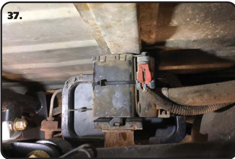
**37.** For trucks with the emissions control on the gas tank crossmember, we attached it to the end of the charcoal canister.
