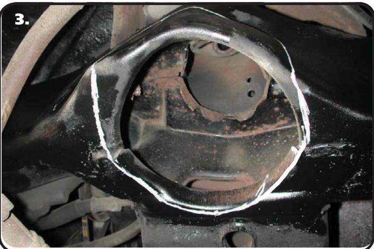
3. To allow clearance for the Shockwave, some trimming may need to be done on the inside of the coil spring pocket as shown by the white line in the picture. This is best done with either a cut off wheel or plasma cutter. Grind all cuts smooth when finished.
