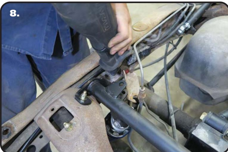
8. Use a saw-z-all or cut off tool to cut the brake line bracket flush with the inside edge of the frame rail.
