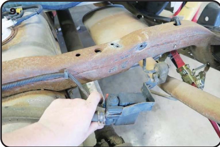
9. If your truck came equipped with the emissions module mounted at the center of the gas tank crossmember, it will need to be relocated. The emissions control locations vary through the years. If the differential vent is mounted on top of the crossmember, it can be moved to the mounting hole for the emissions control module.
