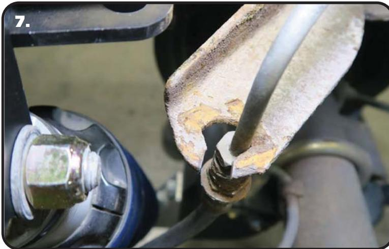
7. To keep from opening the brake line, we cut a notch in the end of the brake line bracket to slide the brake line through.
