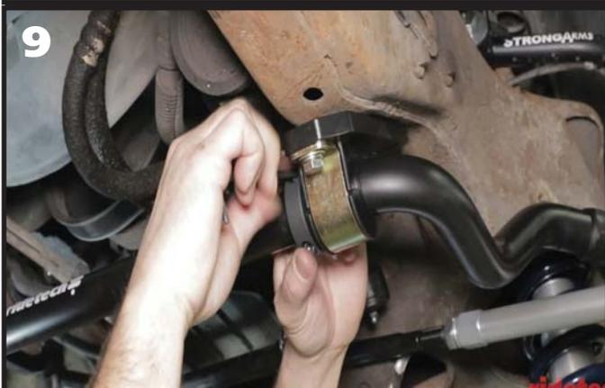
**9.** Torque the SwayBar mounting hardware to 30 ftlbs. Install the locking rings on the inside of each bushing assembly. Use a hex key to take the locking ring apart. Reassemble it on the bar positioned next to the inside of the bushing assembly. Push the locking ring up against the bushing assembly and tighten.
