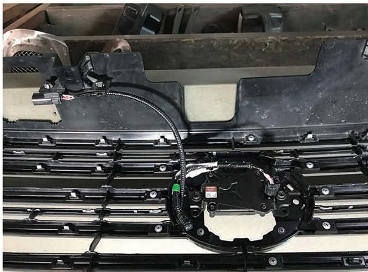
3. Remove TSS sensor module and harness from factory grille.
