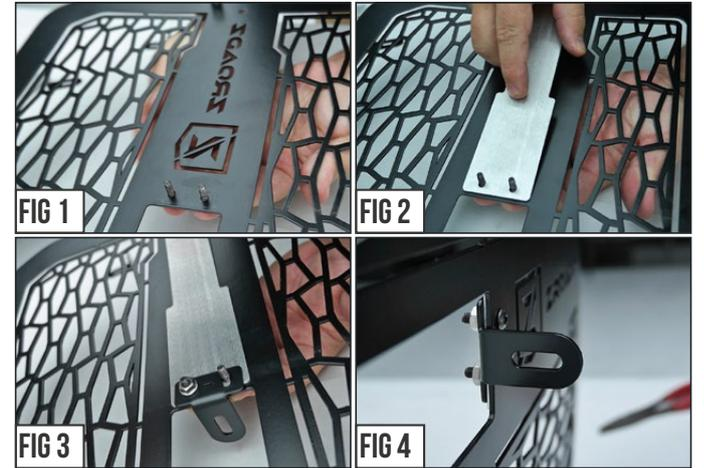
**STEP 2** Put into place one of the Bracket Tabs and secure with provided Hardware as seen in Fig. # 1-4.
