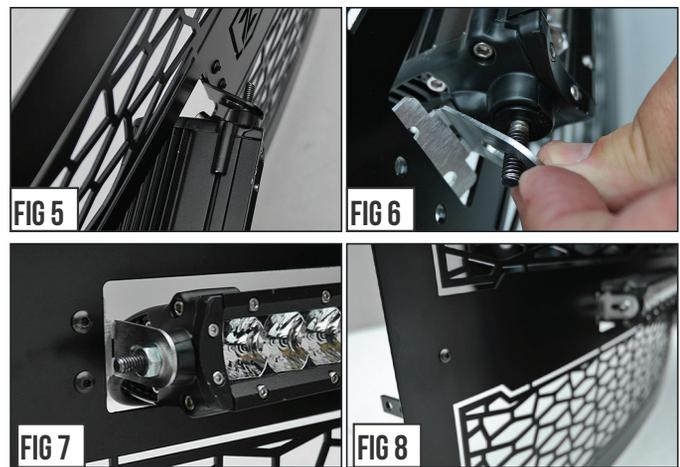
**STEP 3** From the face side of grille slip the LED Light bar into place. On the opposite side, position the remaining bracket and finally tighten LED and Brackets into position.
