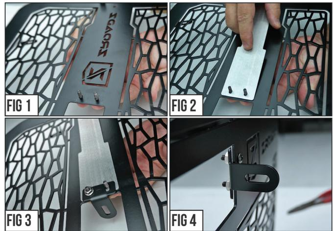
**STEP 2** Put into place one of the Bracket Tabs and secure with provided Hardware as seen in Fig. # 1-4.
