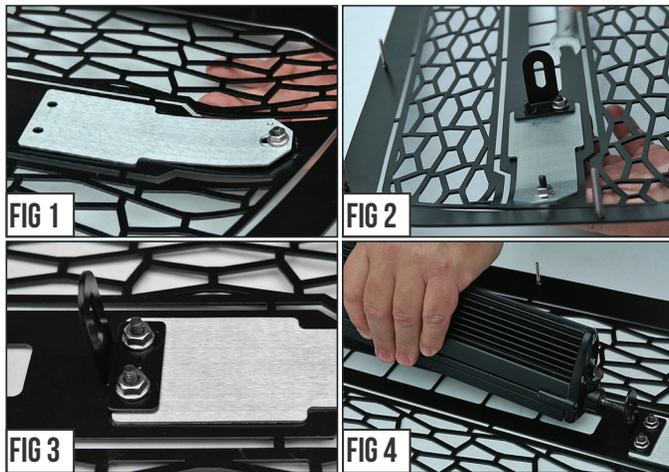
**STEP 2** Put into place one of the Bracket Tabs and secure with provided Hardware as seen in Fig. # 2-4 and then from the backside of grille position LED Light Bar.
