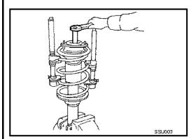
1.) Set the shock absorber in a vise, then loosen (without removing) the piston rod lock nut as shown.
