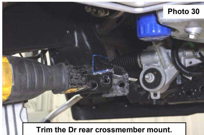
36. Remove the cut portion of the rear crossmember mount. Sand and paint the cut edge to prevent rust. **See Photo 31.**
